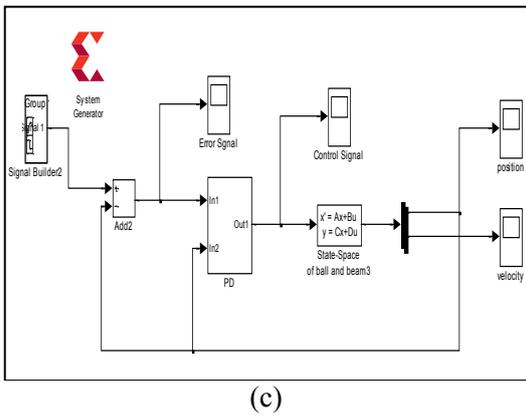
Figure 10: Matlab simulink connection for ball and beam system with PD controller; (a): continuous connection; (b): discrete connection; (c): FPGA connection
