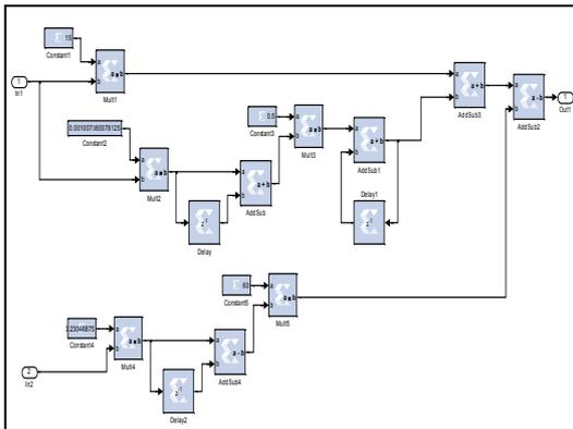
Figure 7: FPGA design of the suggested PID controller
