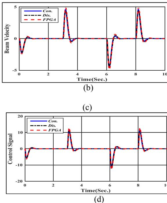
**Figure 15: Simulation and hardware results for complete system (ball and beam system controlled by servo motor) in (continuous, discrete, FPGA) form with step input of mag.0.5: (a) beam position; (b) beam velocity; (c) error signal; (d) servo control signal**
