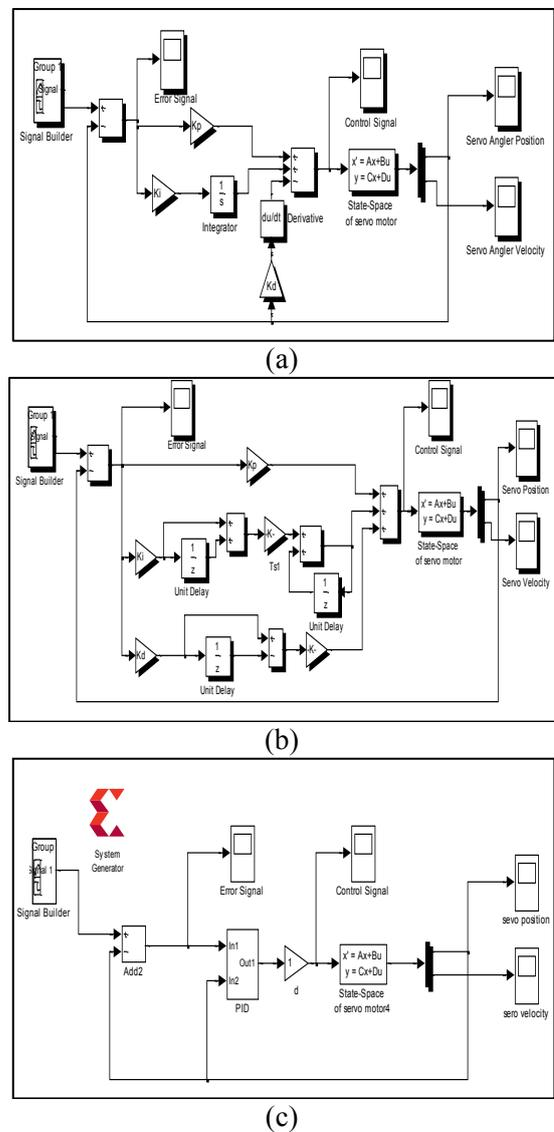
Figure 12: Matlab simulink connection for servo motor system with PID controller; (a): continuous connection; (b): discrete connection; (c): FPGA connection
