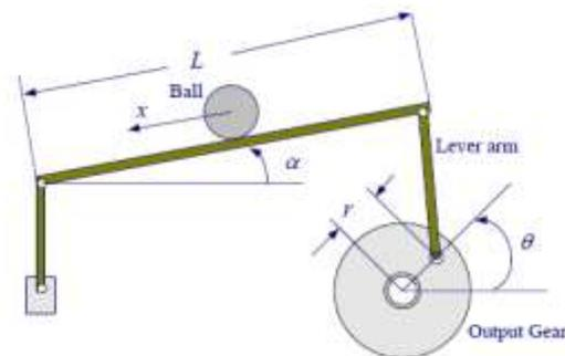
**Figure 2: Schematic of the ball and beam system**
