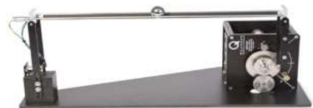
**Figure 1: Real ball on a beam system**
