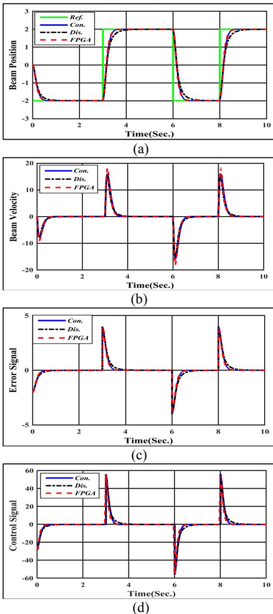
Figure 11: Simulation results for ball and beam system without servo motor controlled by PD in
