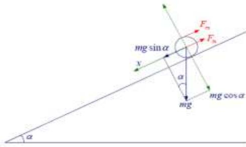
Figure 3: Rolling ball free-body diagram
