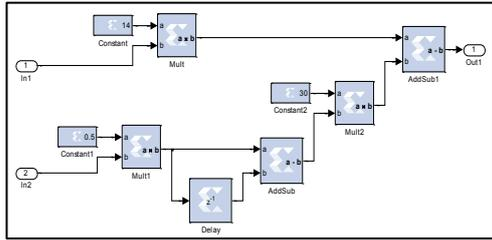
Figure 6: FPGA design of the suggested PD controller
