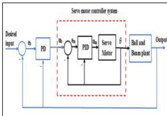
**Figure 4: The block diagram for complete controller for ball and beam system**
