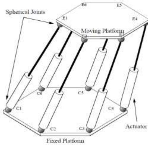
Figure (1) Gough-Stewart mechanism
