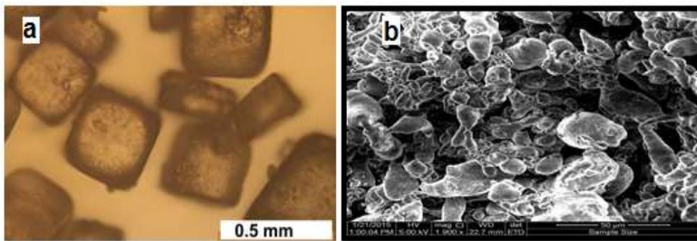
**Figure (1): Morphology of (a) NaCl particles by optical microscope, (b) Al powder by SEM.**
