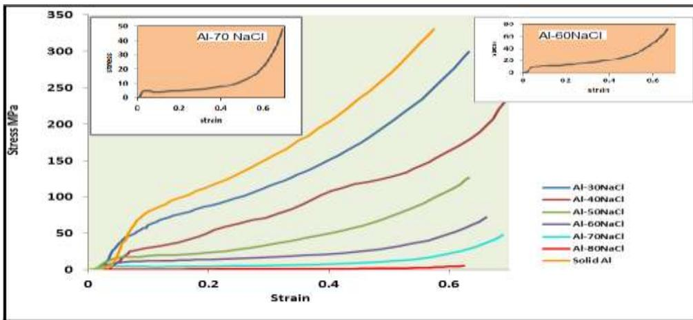
Figure (4): Compressive stress-strain curves of aluminum foam with different NaCl content.
