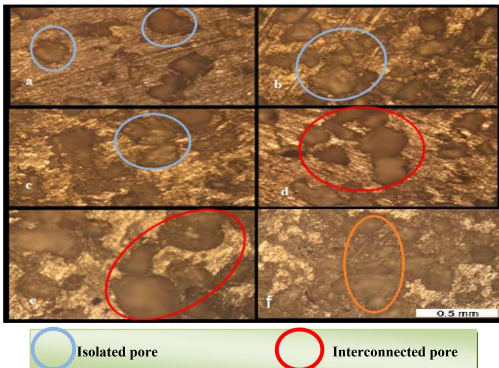
Figure (4): Optical micrograph of samples with different NaCl content; a) Al-30NaCl, b) Al-40NaCl, c) Al-50NaCl, d) Al-60NaCl, e) Al-70NaCl, f) Al-80NaCl
