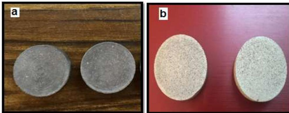
Figure (2): Aluminum specimens (a)after sintering, (b) after dissolution process.
