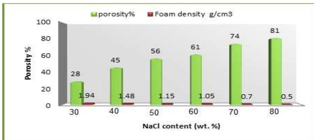
Figure (3): The effect of NaCl content on porosity and foam density.
