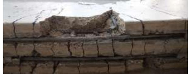
Figure 13: debonding of CFRP bars
