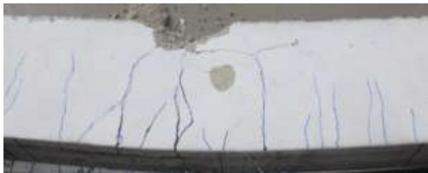
Figure 9: Concrete crushing in RL beam
