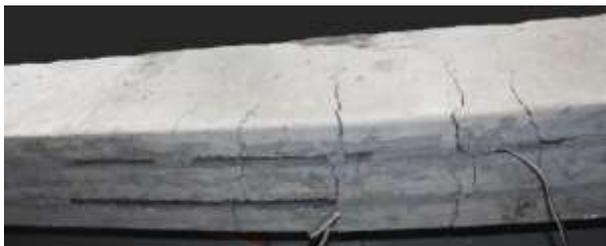
Figure 7: Failure mode with debonding of fiber in SL beam
