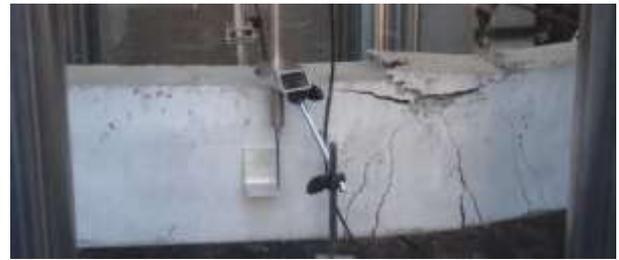
Figure 12: concrete crushing in RB beam
