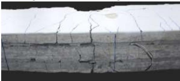
Figure 10: Failure mode with debonding of fiber in RL beam
