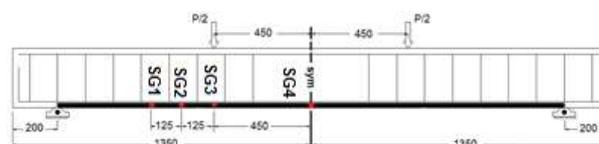
Figure 2: Strain gauge layout
