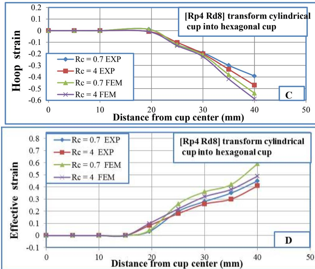
Figure (8) Effect of wall corner radius of die on (A) radial strain (B) thickness strain (C) hoop strain (D) effective strain
