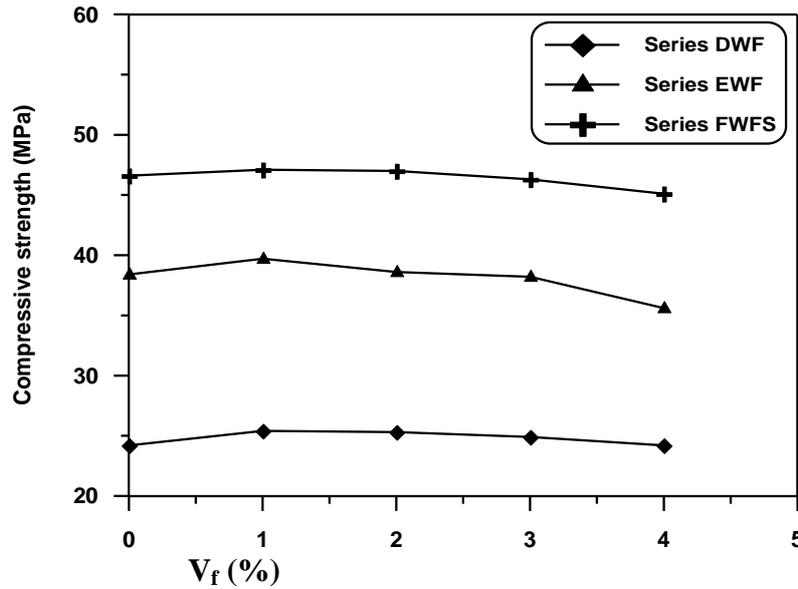
Fig.4: Variation of the 28 day cube compressive strength versus volume percentage of waste flax fibers for different series
