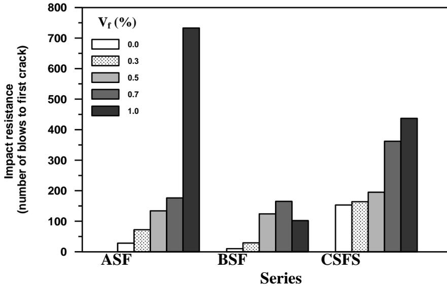
Fig.16: Variation of the 90 day impact resistance at first crack with volume percentage of steel fibers for different series
