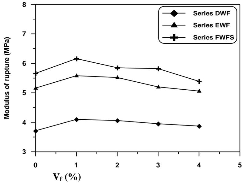
Fig.12: Effect of volume fraction of waste flax fibers on 28 day modulus of rupture for different series
