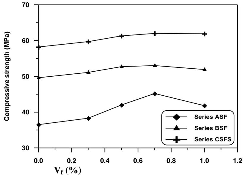
**Fig.3 : Variation of the 90 day cube compressive strength with volume fraction of steel fibers for different series**
