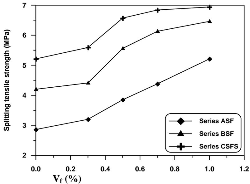
Fig.7: Effect of volume fraction of steel fibers on 90 day splitting tensile strength for different series
