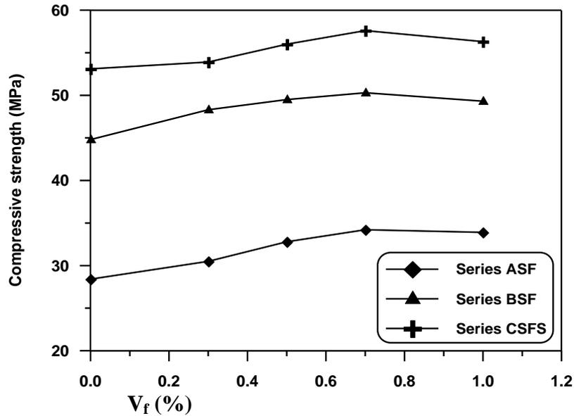
**Fig.2: Variation of the 28 day cube compressive strength with volume fraction of steel fibers for different series**
