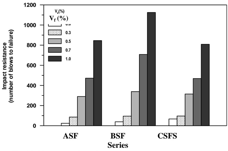
**Fig.15: Variation of the 28 day impact resistance at failure with volume percentage of steel fibers for different series**
