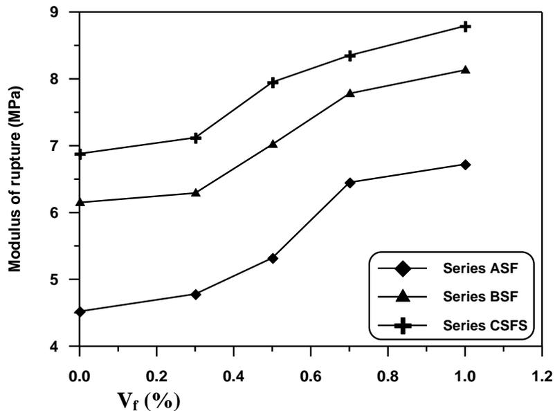
**Fig.11: Effect of volume percentage of steel fibers on 90 day modulus of rupture for different series**
