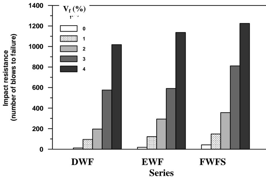
Fig.19: Variation of the 28 day impact resistance at failure against volume fraction of waste flax fibers for different series
