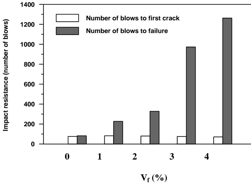
**Fig.20: Variation of the 90 day impact resistance against volume fraction of waste flax fibers for series FWFS**
