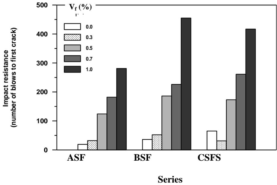
**Fig.14: Variation of the 28 day impact resistance at first crack with volume percentage of steel fibers for different series**
