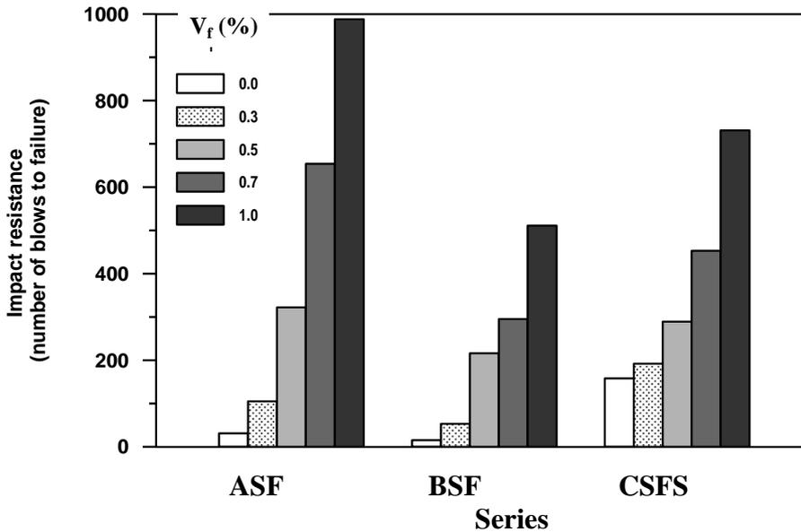
Fig.17: Variation of the 90 day impact resistance at failure with volume percentage of steel fibers for different series
