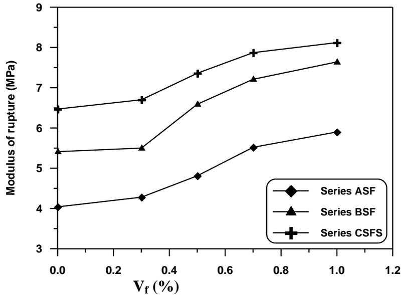
**Fig.10: Effect of volume percentage of steel fibers on 28 day modulus of rupture for different series**
