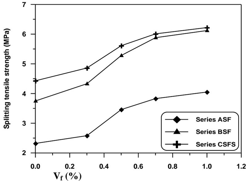
Fig.6 : Effect of volume fraction of steel fibers on 28 day splitting tensile strength for different series
