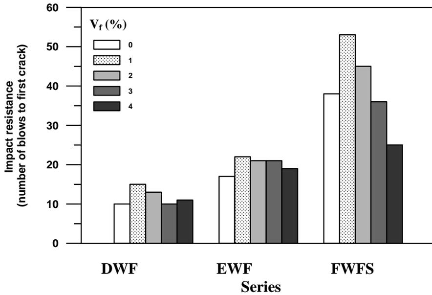
Fig.18: Variation of the 28 day impact resistance at first crack against volume fraction of waste flax fibers for different series
