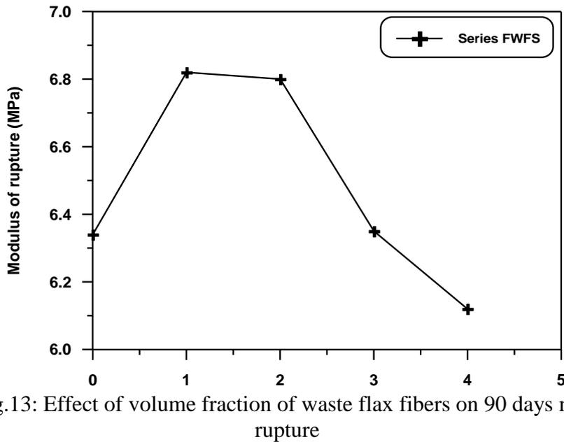
Fig.13: Effect of volume fraction of waste flax fibers on 90 days modulus of rupture
