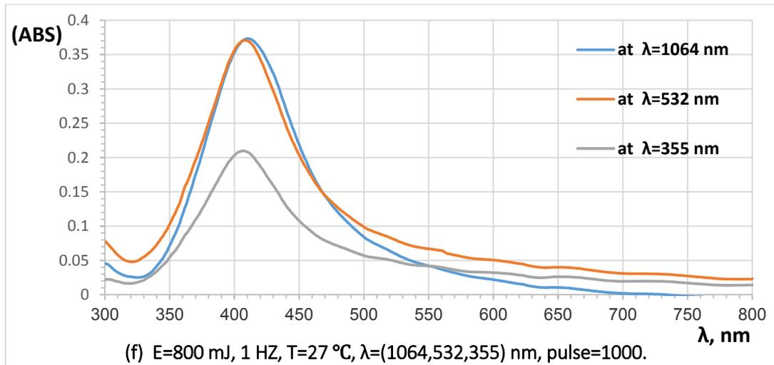
Figure (6): shows the UV–Vis absorption spectra for silver nanoparticles prepared using PLAL synthesis at E= 800 mJ, λ= (1064, 532, 355) nm, 1 HZ, T= 27 °C and pulses numbers (a) 500, (b) 600, (c) 700, (d) 800, (e) 900, (f) 1000.
