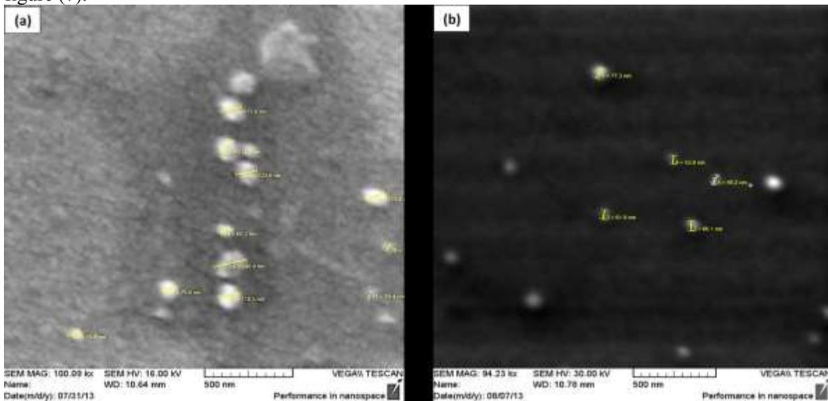
Figure (7): SEM images of colloidal silver-NPs by PLAL method prepared at 1000 pulses, T=27 °C and different wavelengths (a) 1064 nm and (b) 532 nm.
