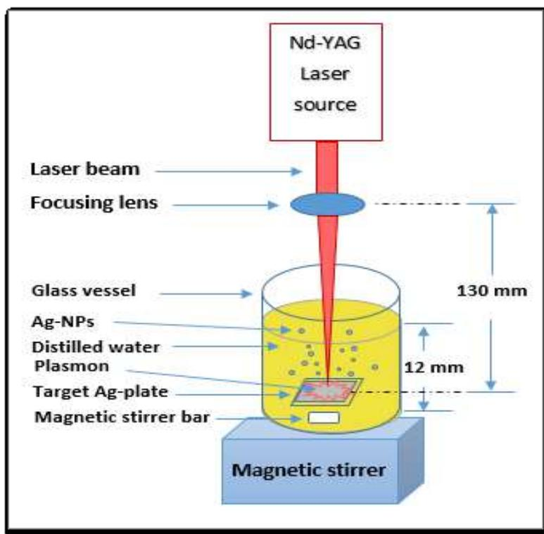
**Figure (1) shows Experimental set up for nanoparticles synthesis, by pulse laser ablation in liquid PLAL technique.**
