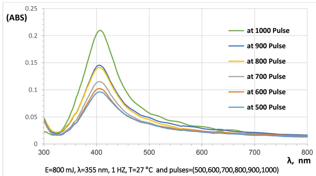
**Figure (4): Shows the UV–Vis absorption spectra for silver nanoparticles prepared using PLAL synthesis at E= 800 mJ,  $\lambda=355$  nm, 1 HZ, T= 27 °C and different pulses numbers.**
