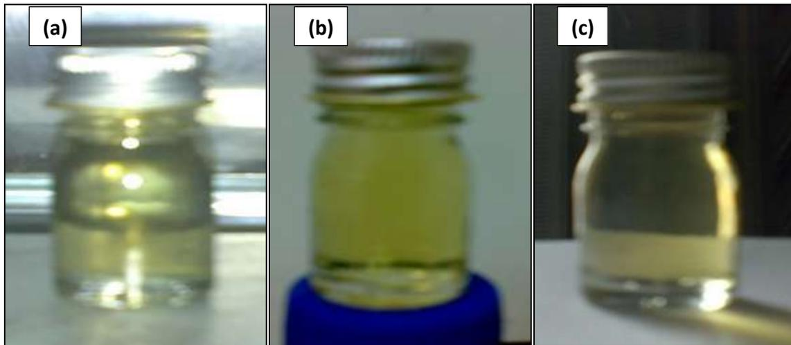
Figure (9): shows images of colloidal silver nanoparticles obtained by PLAL at 1000 pulse and (a)  $\lambda$ = 1064 nm, (b)  $\lambda$ = 532 nm, (c)  $\lambda$ = 355 nm.
