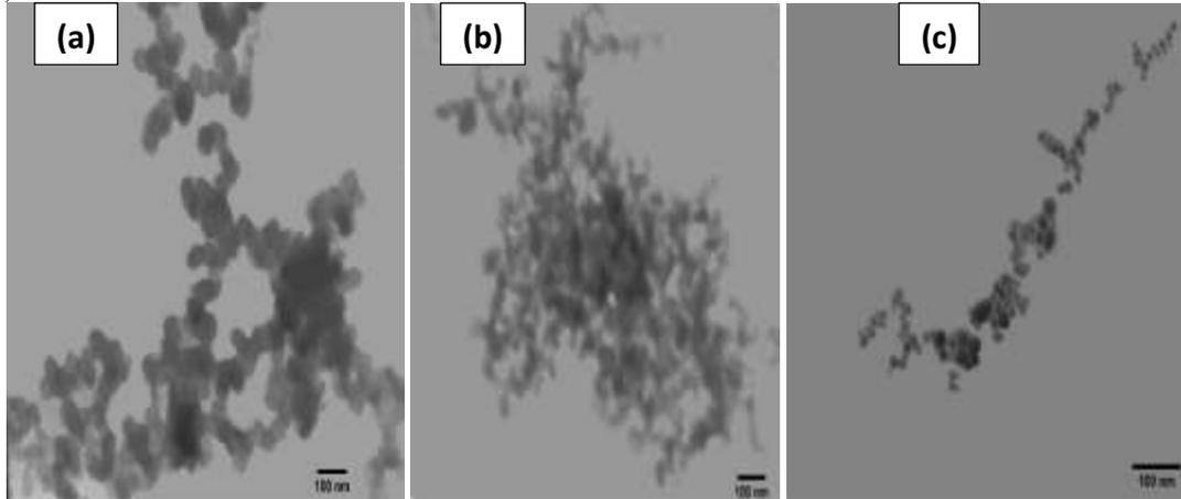
Figure (8): Shows TEM image for colloidal silver nanoparticles prepared by PLAL, at E= 800 mJ, 1 HZ, T= 27 °C, 1000 pulse and (a) at  $\lambda$  =1064 nm, average size of the particles is (55-60) nm, (b) at  $\lambda$  =532 nm, average size of the particles is 35-40 nm, (c) at  $\lambda$  =355 nm, average size of the particles is 28 nm.
