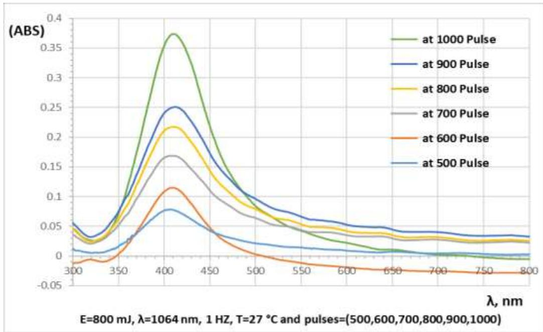
Figure (2) Shows the UV–Vis absorption spectra for silver nanoparticles prepared using PLAL synthesis at  $E= 800 \text{ mJ}$ ,  $\lambda=1064 \text{ nm}$ ,  $1 \text{ HZ}$ ,  $T= 27 \text{ }^\circ\text{C}$  and different pulses numbers.
