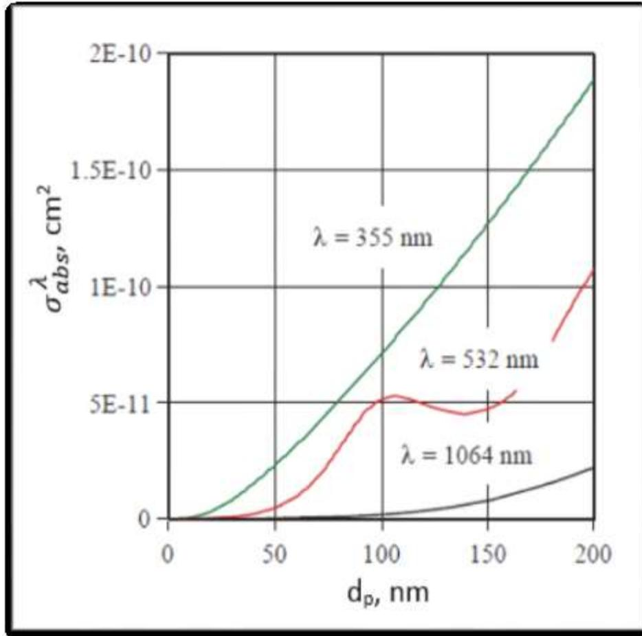
Figure (5): Absorption cross sections,  $\sigma_{abs}^{\lambda}$ , for spherical silver nanoparticles calculated as a function of particle diameter,  $d_p$ , with Mie theory [12,13] for three characteristic wavelengths of Nd:YAG laser.
