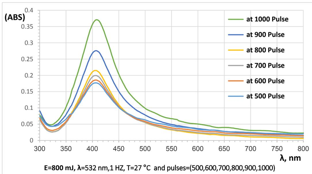
Figure (3): Shows the UV–Vis absorption spectra for silver nanoparticles prepared using PLAL synthesis at  $E= 8400 \text{ mJ}$ ,  $\lambda=532 \text{ nm}$ ,  $1 \text{ HZ}$ ,  $T= 27 \text{ }^\circ\text{C}$  and different pulses numbers.
