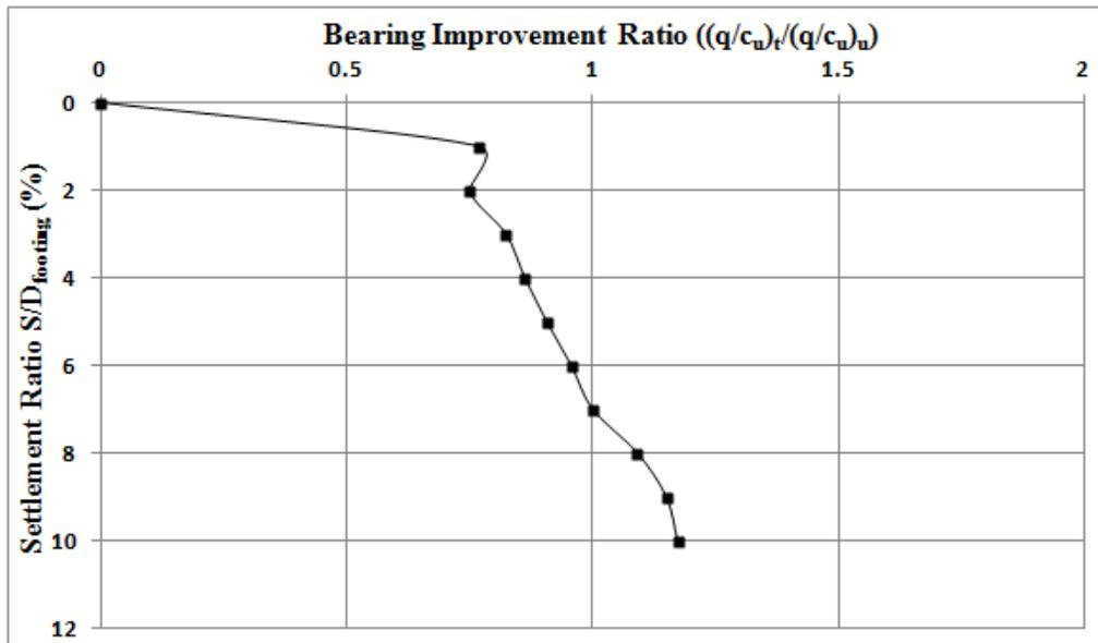
Figure (5) Bearing improvement ratio versus settlement ratio for soft soil treated with sand columns.
