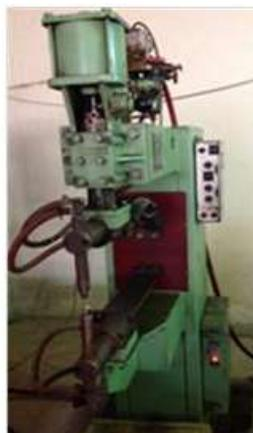
Figure (2) Spot welding machine
