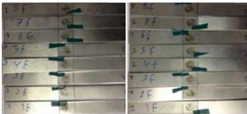
**Figure (3) the welded specimen**
