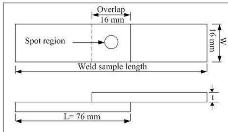
Figure (1) Overlapping of two welded plates
