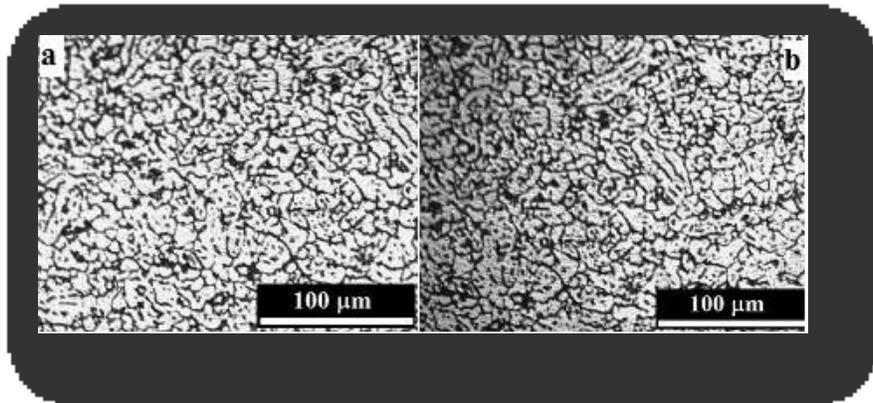
Figure (24) Microstructure of similar joint of AA 6061-T6, (a)  $t = 0.5$  mm (b)  $t = 0.7$  mm
