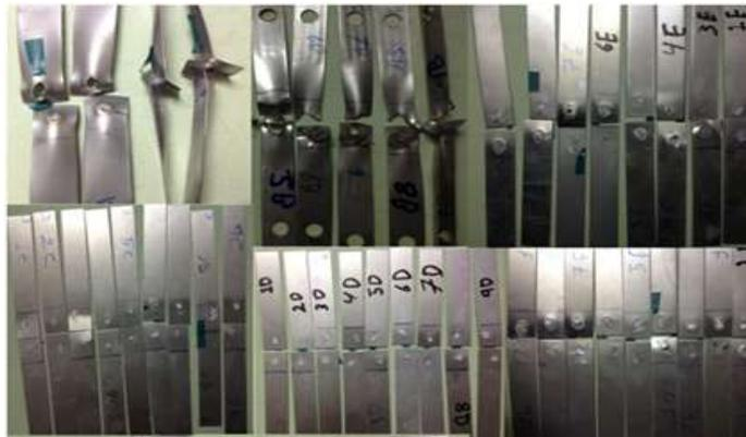
Figure (5) the tested shear force specimen
