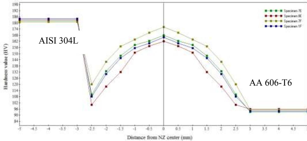
Figure (22) Hardness values of dissimilar joint for (AISI 304L with AA 606-T6)
