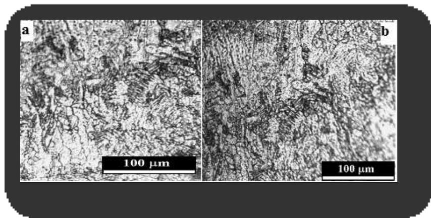
Figure (23) Microstructure of similar joint of AISI 304L, (a) t = 0.5 mm (b) t = 0.7 mm
