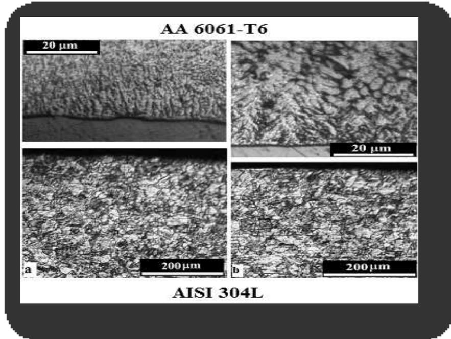
Figure (25) Microstructure of dissimilar joint of AISI 304L with AA 6061-T6,
