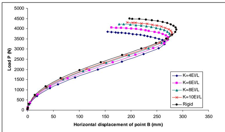
Figure. (21) Effect of joint stiffness on post buckling behavior in terms of load-horizontal displacement of point B of one-bay two-story steel frame
