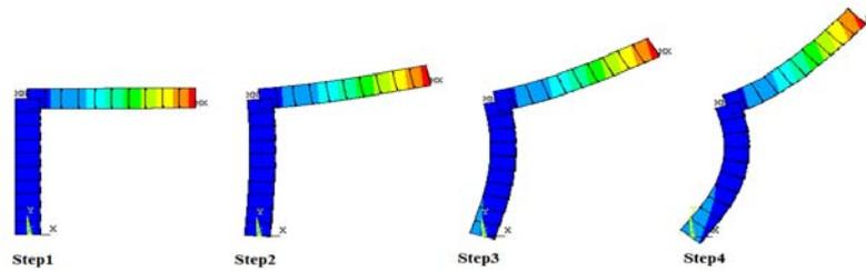
Figure. (9) post buckling behavior of Lee's frame semi rigid connection in different load steps
