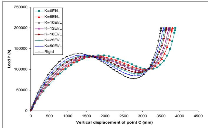
Figure. (15) Effect of joint stiffness on post buckling behavior in terms of load-vertical displacement of point C of one- bay one-story steel frame
