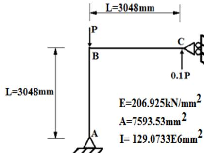
Figure (3) Geometry , loading and section properties of Lee's frame
