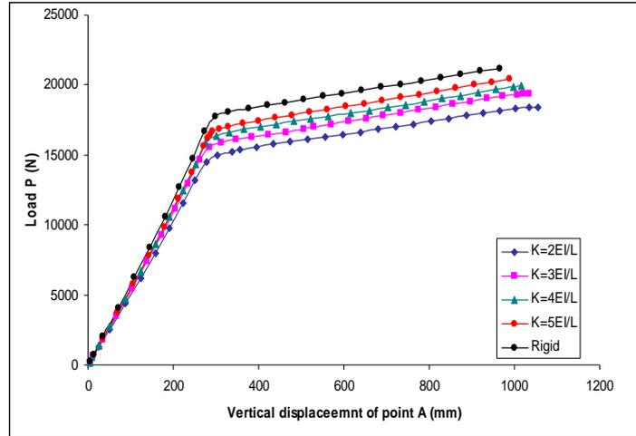
Figure. (26) Effect of joint stiffness on post buckling behavior in terms of load-vertical displacement of point A of three-bay two-story frame
