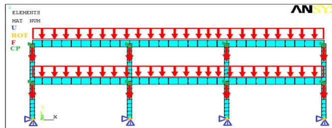
Figure.(25) Modeling three-bay two-story frame in ANSYS
