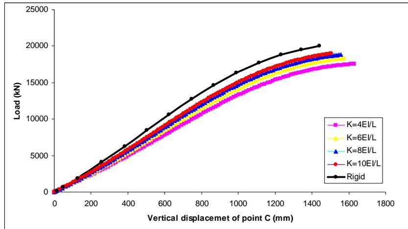
Figure.(8) Effect of spring stiffness value (semi rigid connection ) on load-vertical displacement of point C for Lee's frame
