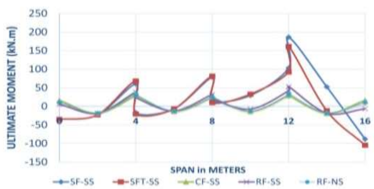
Figure (28): Settlement case 2-UM in GFB along axis A for different type of footings
