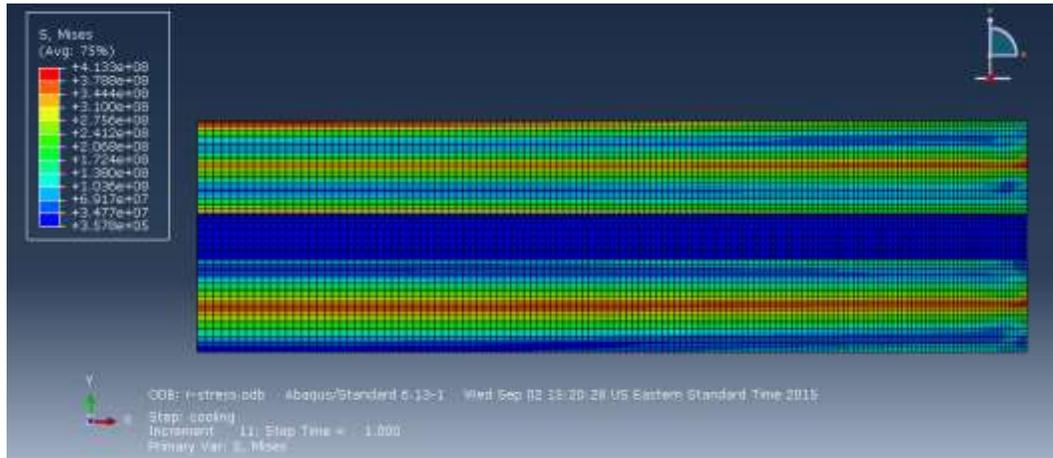
**Figure (7):Nucleated stresses at free edge in case (n=1) under service conditions**
