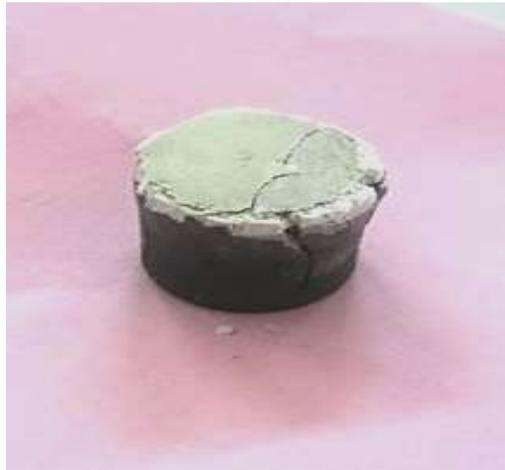
**Figure (11) Crashed stepwise FGM specimen**
