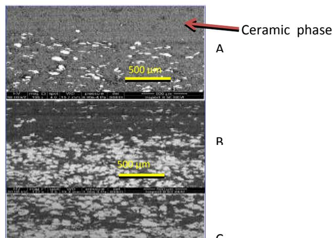
**Figure (9) SEM image of stepwise FGM**
