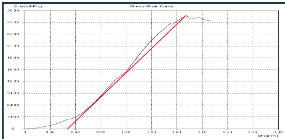
**Figure (10): Stress-strain curve of compression test**
