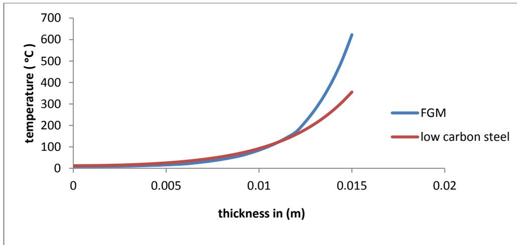
Figure (8):Temperatures distribution across the FGM thickness
