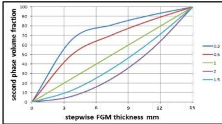
**Figure (2): Stepwise FGM with different (n) values**
