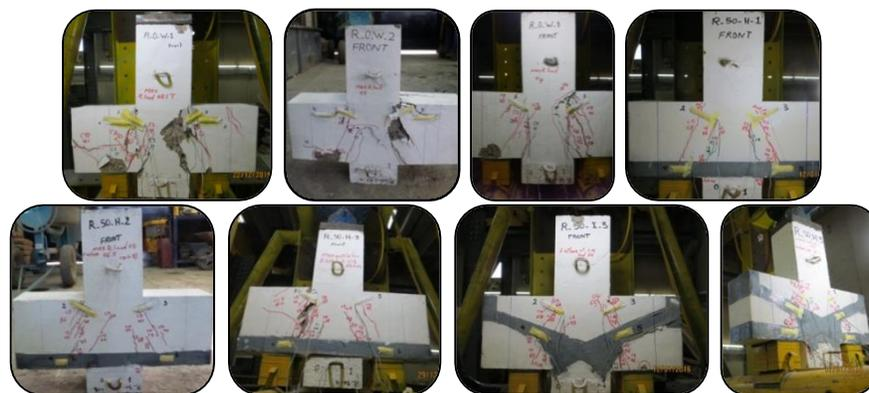
Figure 8 - The Crack pattern and Mode of Failure for the Non-Reversed Repeated Loaded Specimens
