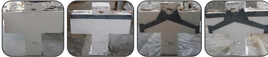
Figure 2 - Photos of Plain and 50-mm Strengthened Specimens
