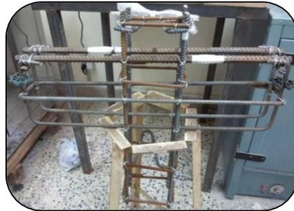
**Figure 17 - Locations of Steel Strain Gauges**
