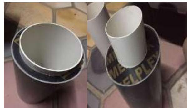
**Figure 3: Molds of the tested specimens**
