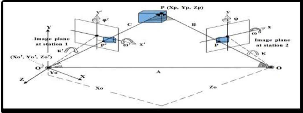
Figure (7): Coplanarity Condition [2]
