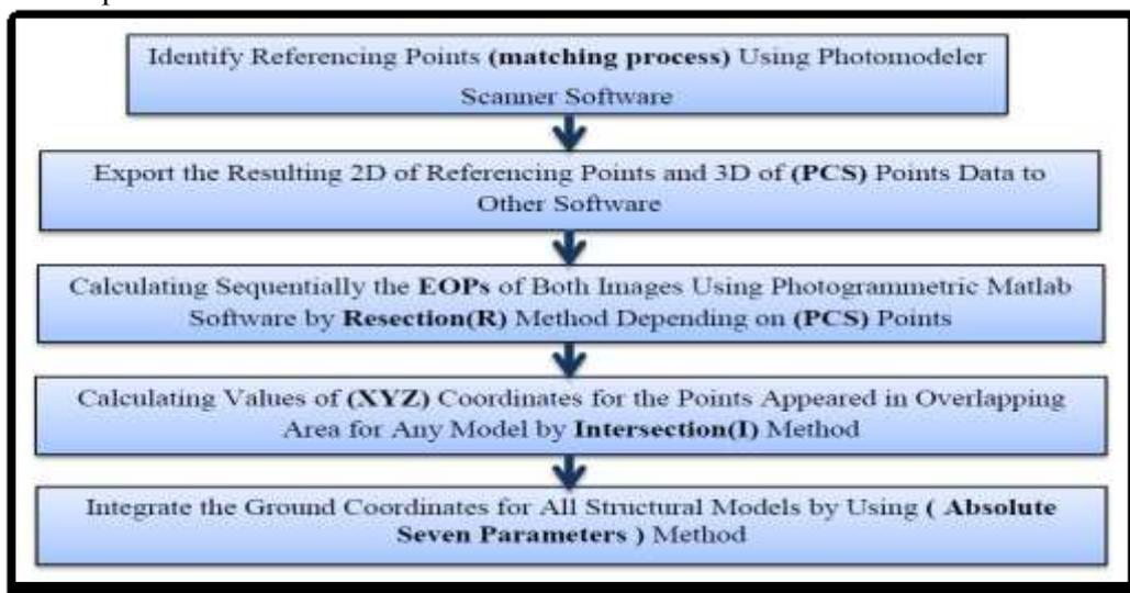
Figure (5): 3D Coordinates of the Structure – Flow Chart
