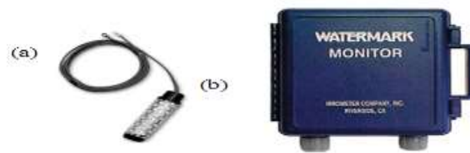
Figure(2).suction measurement: a) watermark sensor, b) watermark monitor.
