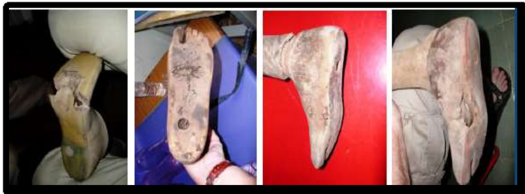
Figure (1) Failure prosthetic foot including tore foot region.
