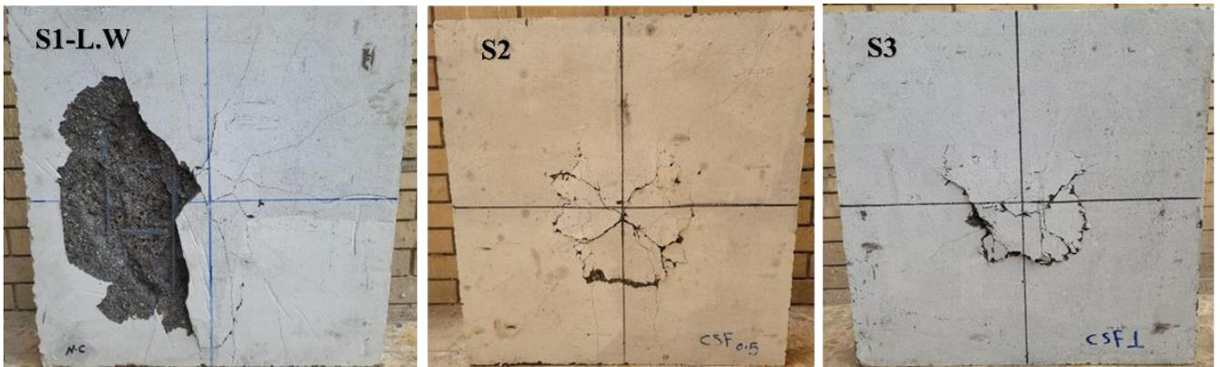
**Fig. 13.** Modes of failure and crack patterns
