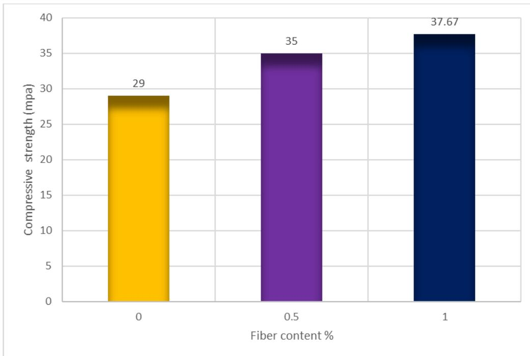
**Fig. 7. Average compressive strength of mixes**
