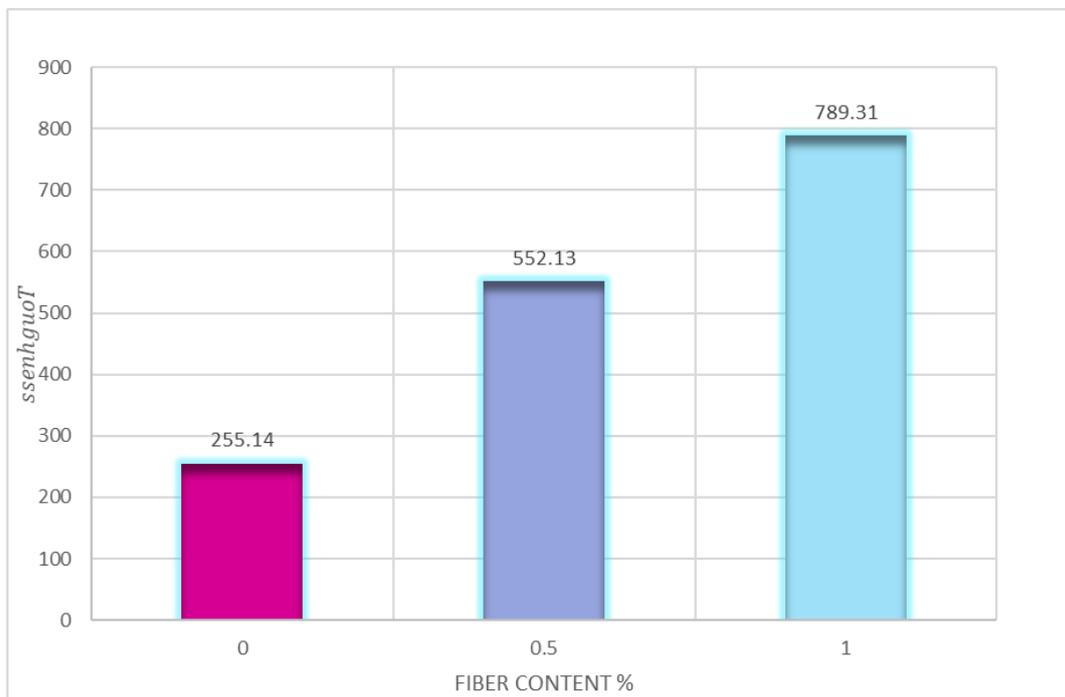
**Fig. 15. Toughness of tested Slab Specimens**
