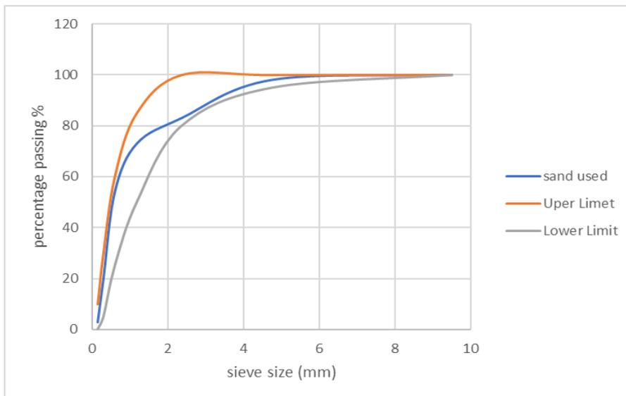
**Fig. 1. Fine aggregate grading curve**
