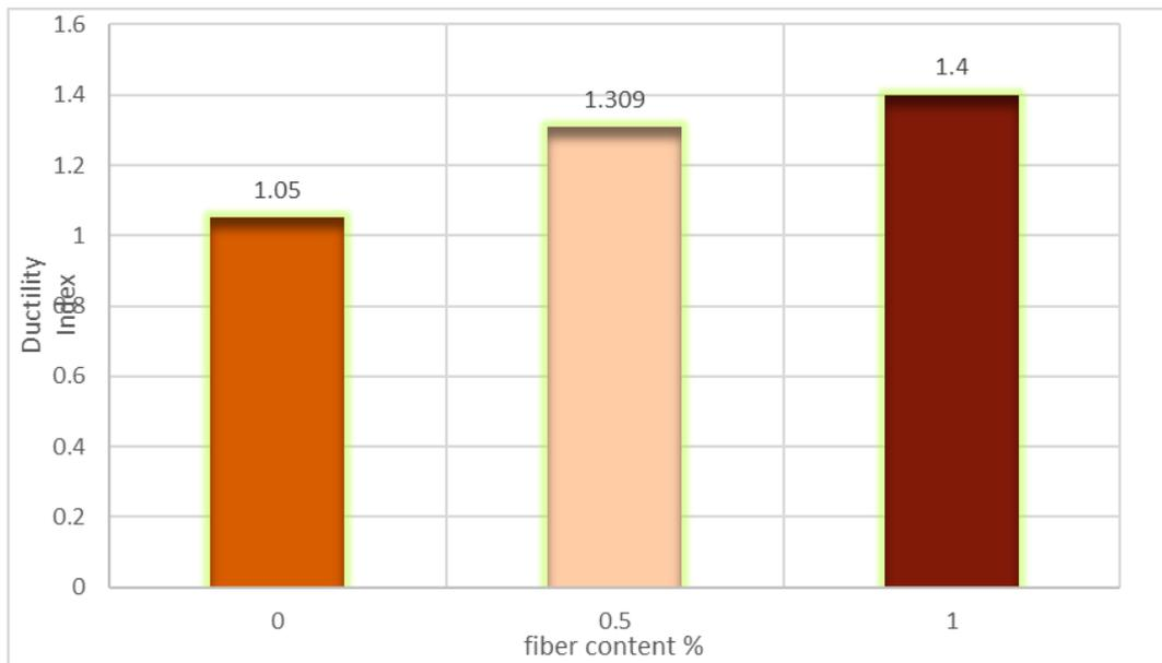
**Fig. 14.** ductility of Tested Slabs
