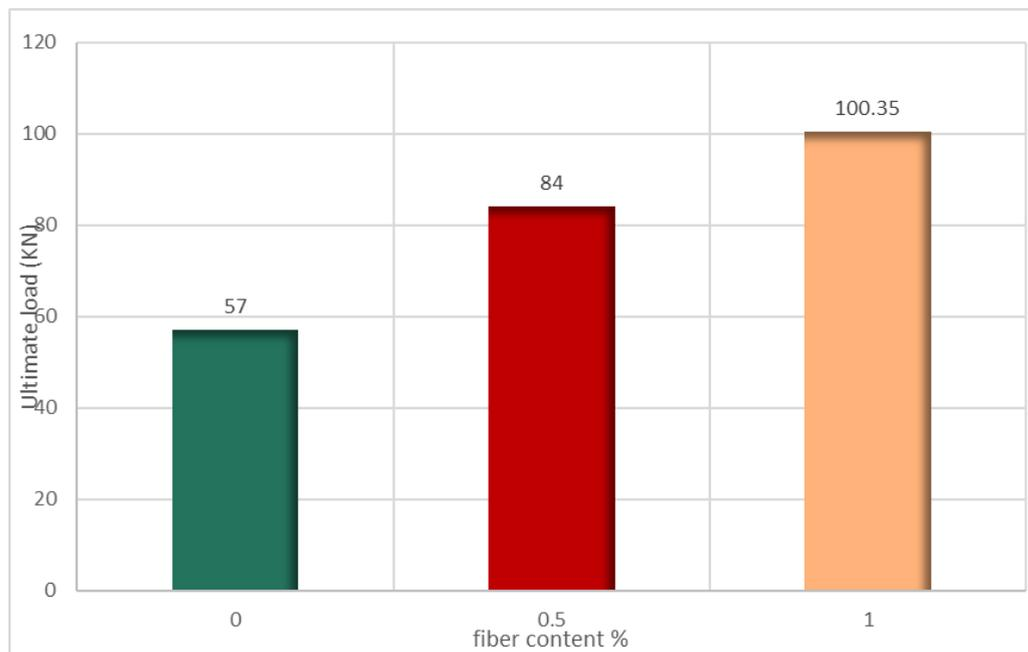
**Fig. 11.** Ultimate punching shear load vs Steel fiber content
