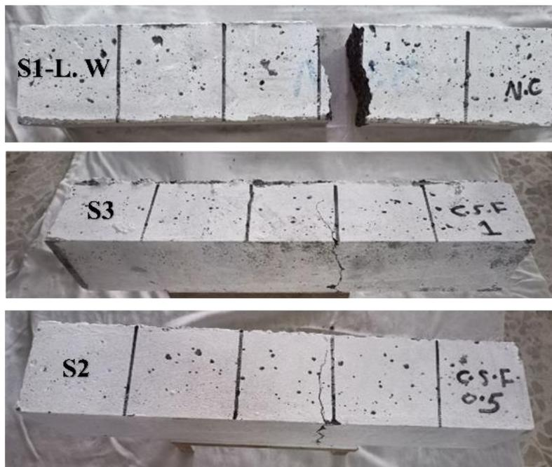
**Fig. 10. Prism specimens and failure shapes**
