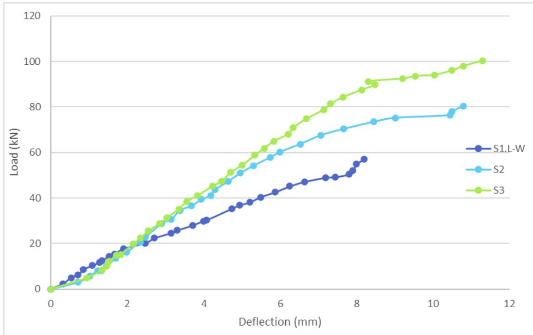
**Fig. 12.** Load- deflection curve for slabs
