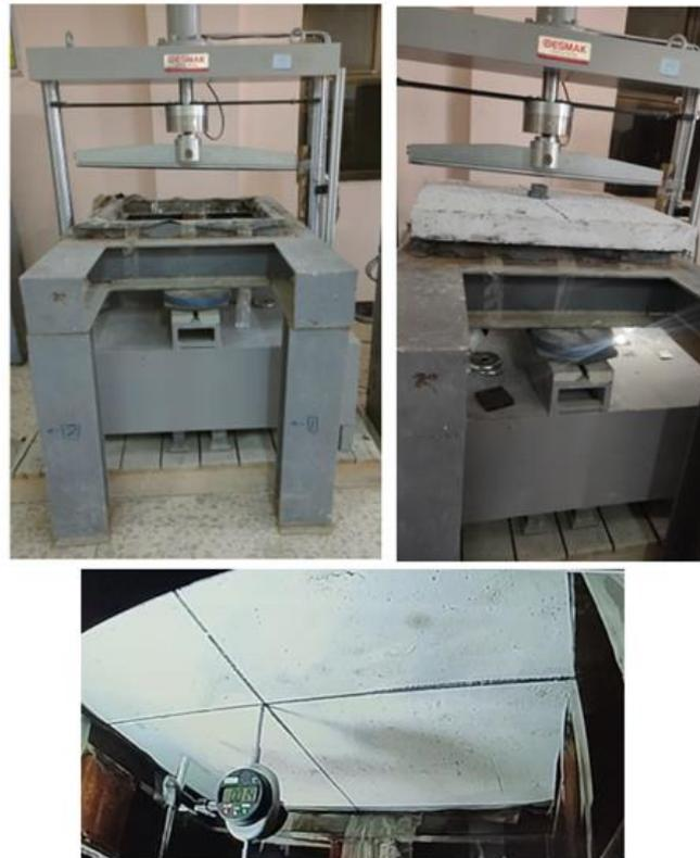
**Fig. 6. Process of punching shear test of slabs**
