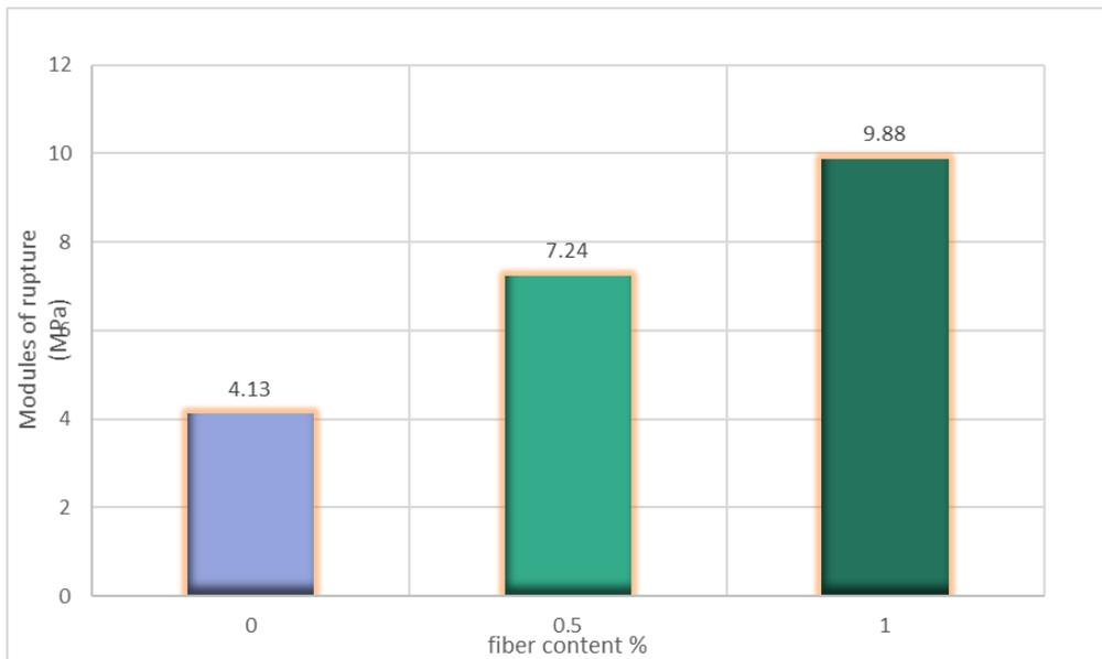
**Fig. 9. Modules of rupture**
