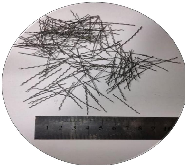
**Fig. 4.** Crimped steel fiber
