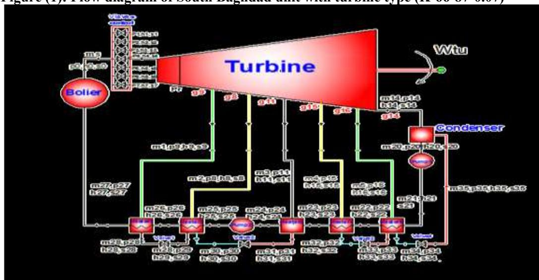
Figure (2): Flow diagram of South Baghdad unit with turbine type (K-55-58.8-0.083)
