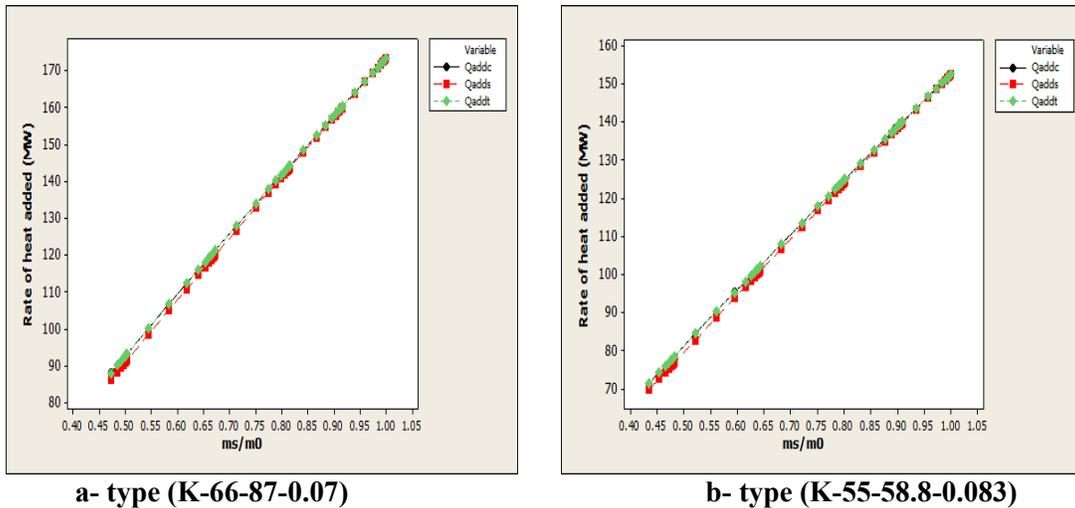
**Figure (6): Variation rate of heat added with flow rate ratio at various types of control for condensing power plant (c: constant pressure with nozzle, s: sliding pressure, t: constant pressure with throttling)**
