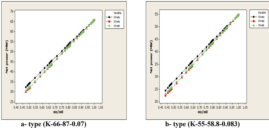
**Figure (5): Variation of net power developed with flow rate ratio at various types of control for condensing power plant (c: constant pressure with nozzle, s: sliding pressure, t: constant pressure with throttling)**
