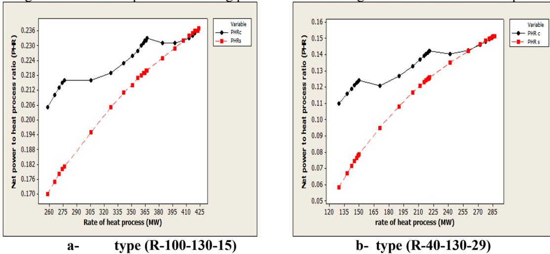
**Figure (14): Variation of net power to heat process ratio with rate of heat process at various types of control for cogeneration power plant (c: constant pressure with nozzle, s: sliding pressure)**
