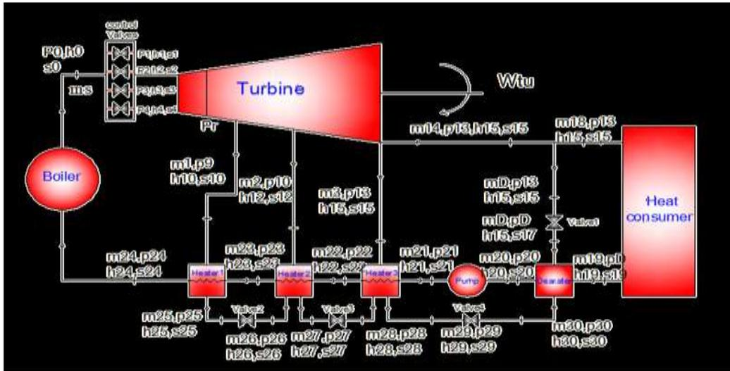
Figure (4): flow diagram of cogeneration plant with back pressure turbine type (R-100-130-15)
