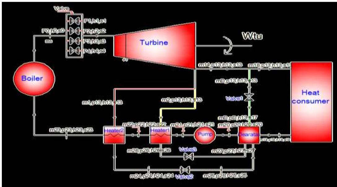
**Figure (3): flow diagram of cogeneration plant with back pressure turbine type (R-40-130-29)**
