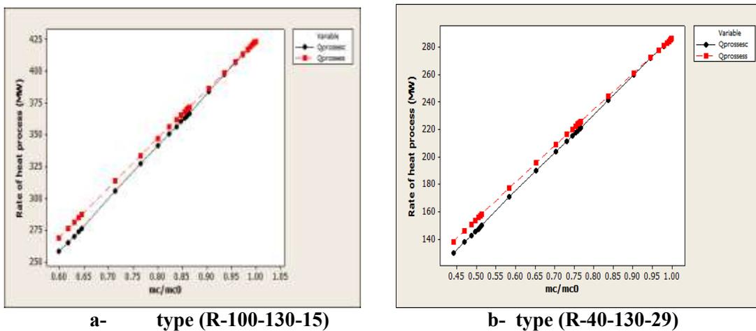
**Figure (13): Variation of rate of heat process with flow rate ratio directed to heat consumer at various types of control for cogeneration power plant (c: constant pressure with nozzle, s: sliding pressure)**
