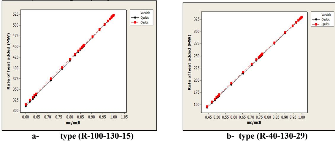
**Figure (12): Variation rate of heat added with flow rate ratio at various types of control for cogeneration power plant (c: constant pressure with nozzle, s: sliding pressure)**
