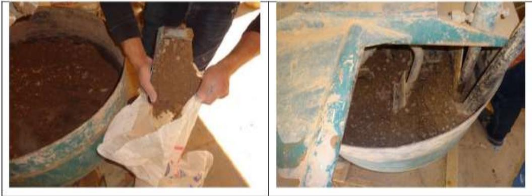
**Figure (7): Preparation of sub base material.**
