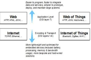
Figure 3: The Position of WoT in OSI Model
