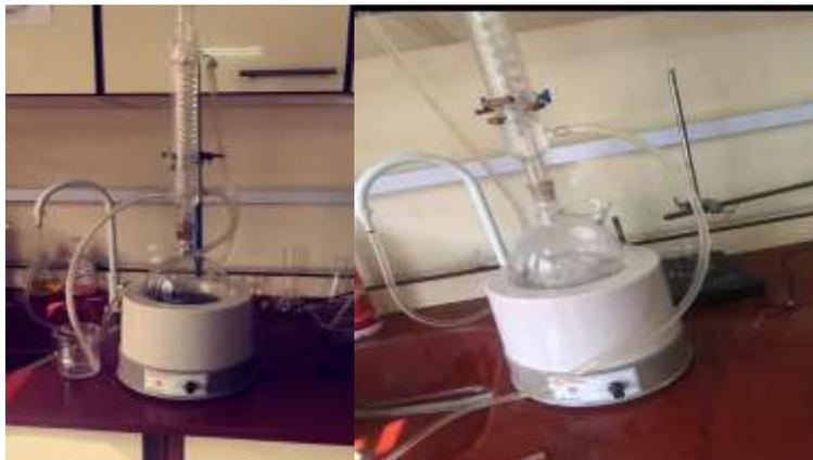
**Figure (1): Reflux apparatus (Close system).**
