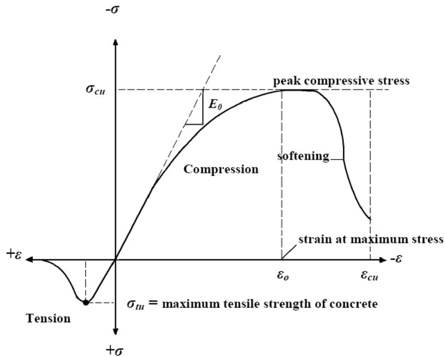
Fig. 4: Typical stress-strain curve for concrete (Kachlakev et al, 2001)
