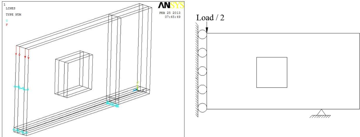
Fig. 8: Half of the beam S08-34-4 is considered due to symmetry
