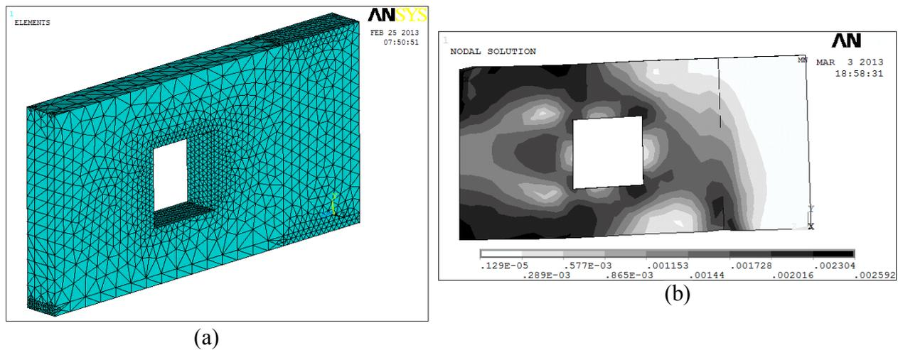
Fig. 9: ANSYS 12.1 model of the beam S08-34-4: (a) finite element mesh, (b) strain intensity
