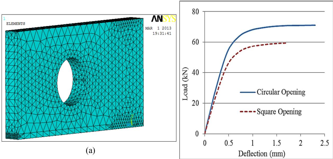
Fig. 11 square vs. circular opening: (a) finite element mesh, (b) load-deflection curves
