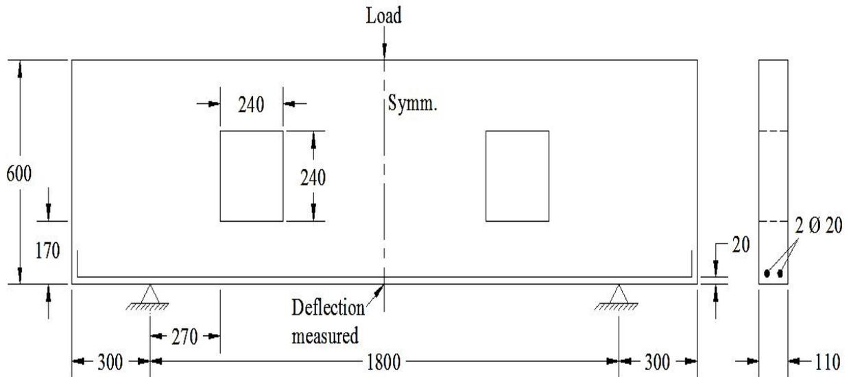
Due to Symmetry; only half of the beam is considered in the ANSYS 12.1 analysis, with the boundary conditions as illustrated in Fig. 8. It is also possible to consider only one quarter of the beam, but this will introduce some complexity on the boundary conditions of the problem.
