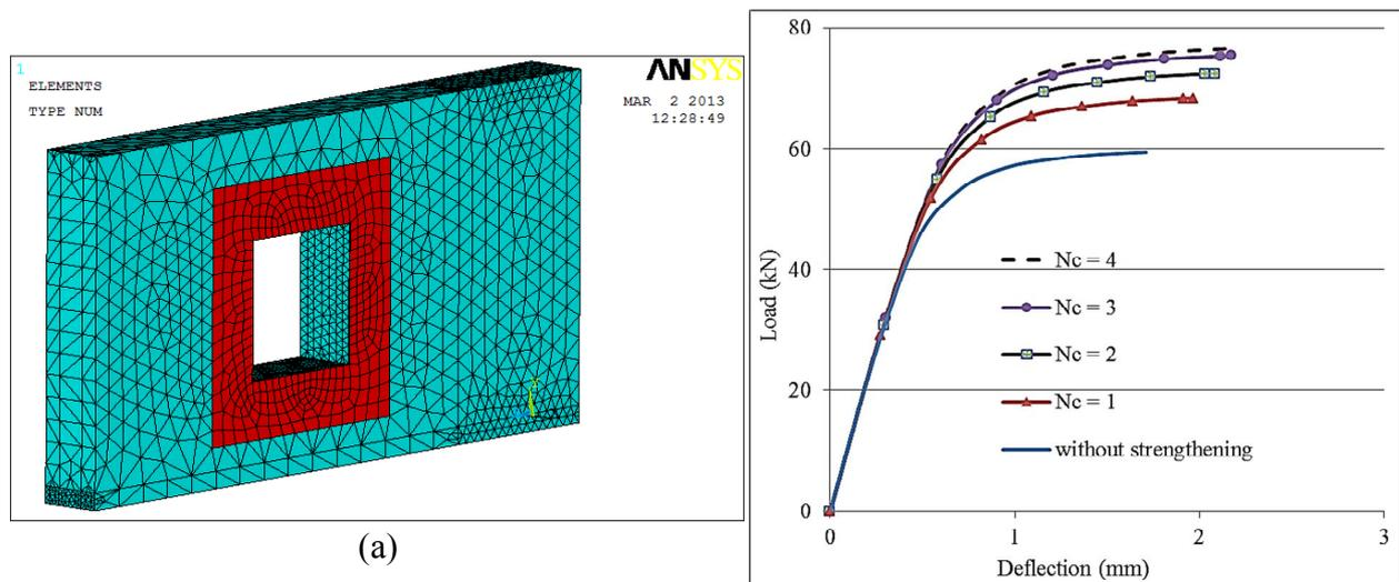
Fig. 12 CFRP laminates around the square opening: (a) finite element mesh, (b) load-deflection curves for several values of  $N_C$
