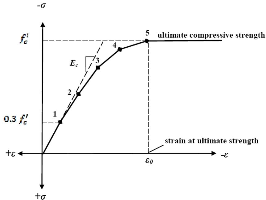
Fig. 5: Simplified compressive stress-strain curve for concrete (Kachlakev et al, 2001)
