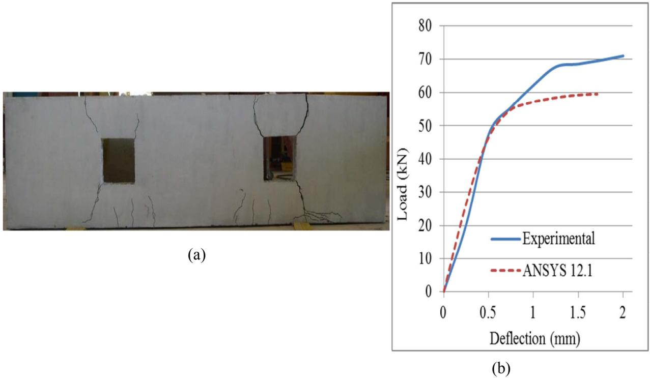
Fig. 10: (a) Crack pattern (Yoo, 2011), (b) Finite element vs. experimental results
