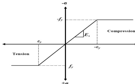
Fig. 6: stress-strain curve for steel bars (Kachlakev et al, 2001)
