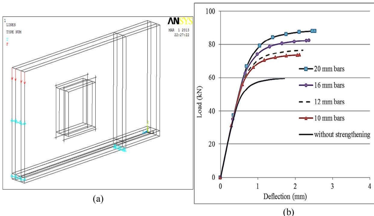
Fig. 13 Steel bars around the square opening: (a) ANSYS 12.1 lines configuration, (b) load-deflection curves for several values of bars diameters
