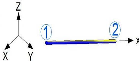
Fig. 2: Geometry of the element SPAR8 (ANSYS 12.1)
