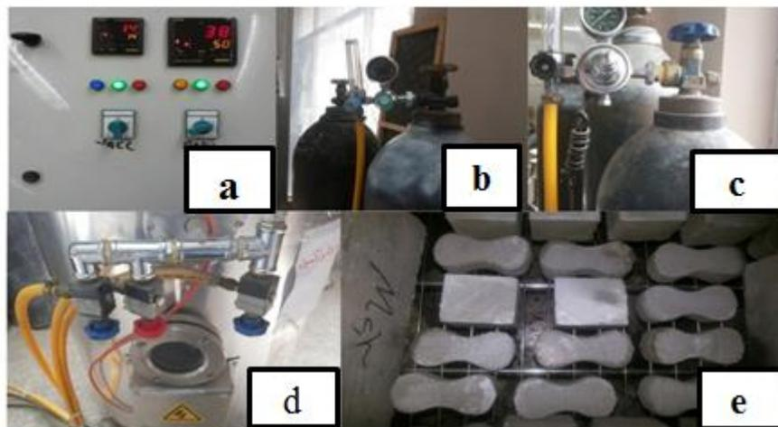
Plate 3: (a): control panel of system, (b): CO<sub>2</sub> bottle supply, (c): O<sub>2</sub> bottle supply, (d): valves of CO<sub>2</sub>, O<sub>2</sub> and vacuum, (e): carbonated specimens.
