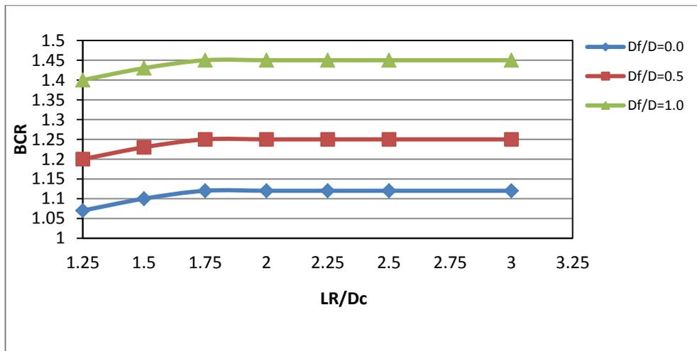
**Figure(11): Bearing capacity ratio(BCR) versus length to diameter ratio (LR/Dc) ,for relative density (RD) 80%**
