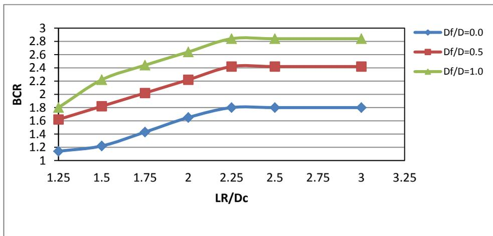
Figure(10): Bearing capacity ratio(BCR) versus length to diameter ratio (LR/Dc) ,for relative density (RD) 60%
