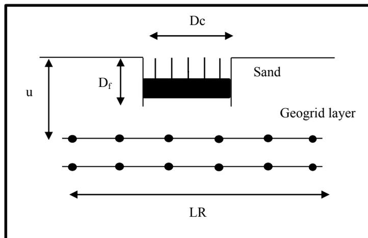
Figure (2) Parameters of circular footing on sand reinforcement
