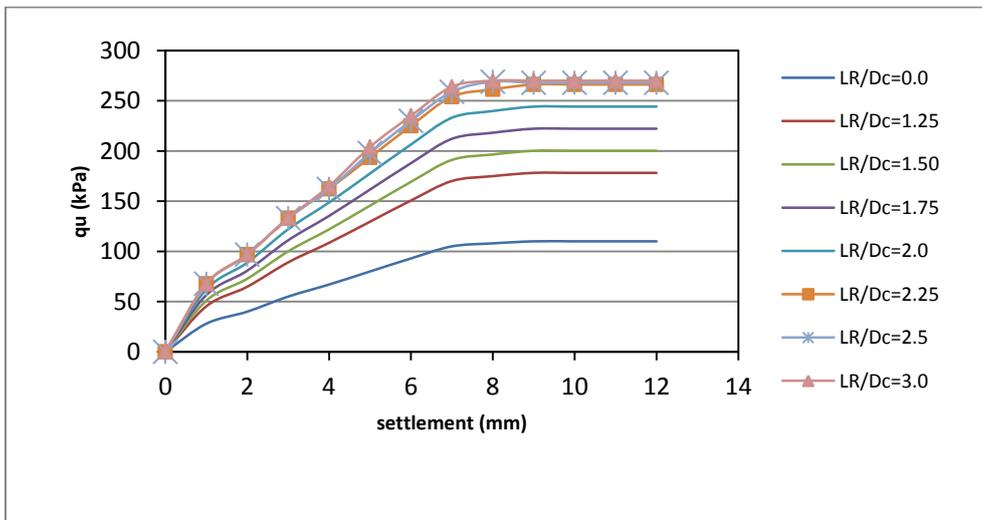
Figure (5): Ultimate bearing pressure – settlement curves for  $D_f/D_c=0.5$ ,  $RD=60\%$
