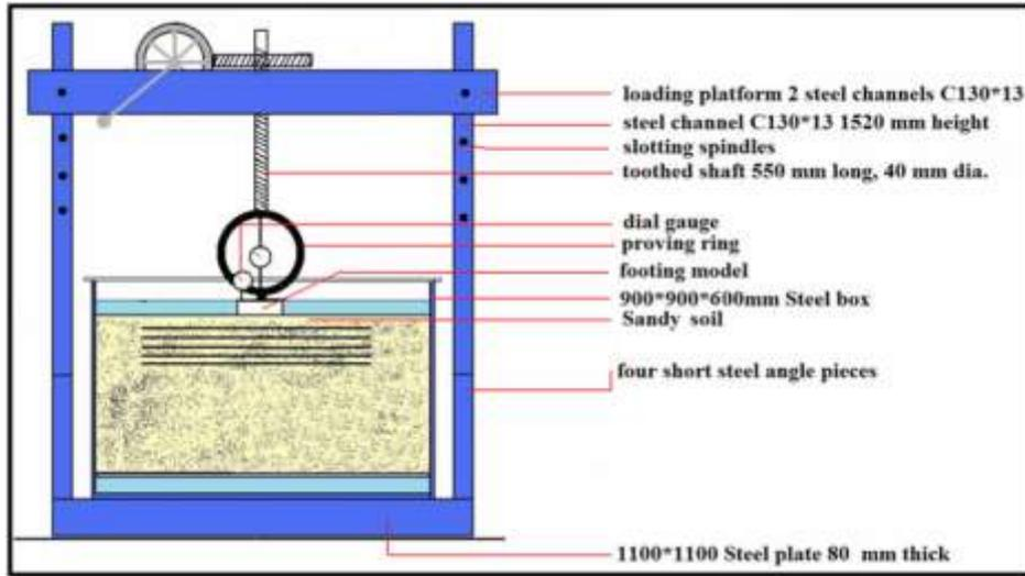
Figure (1) The testing scheme.
