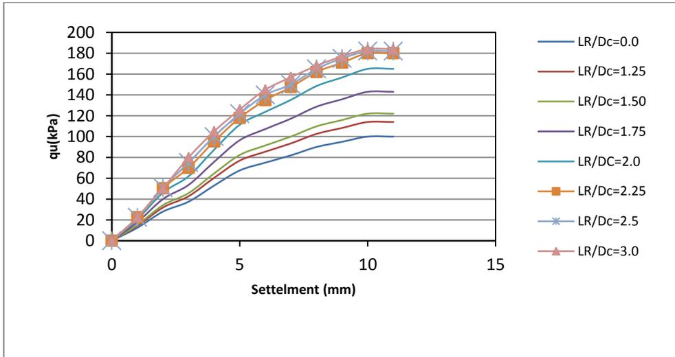
Figure (4): Ultimate bearing pressure – settlement curves for  $D_f/D_c=0.0$ ,  $RD=60\%$
