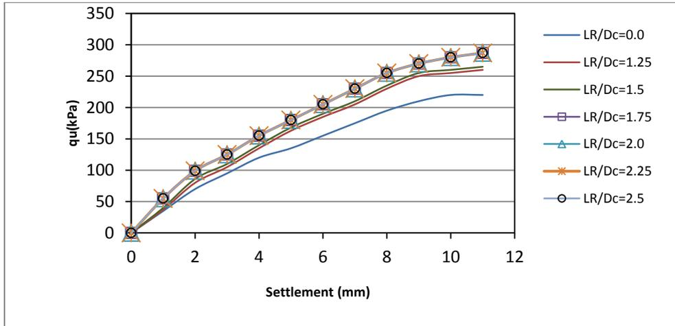
Figure (8): Ultimate bearing pressure – settlement curves for  $D_f/D_c=0.5$ ,  $RD=80\%$
