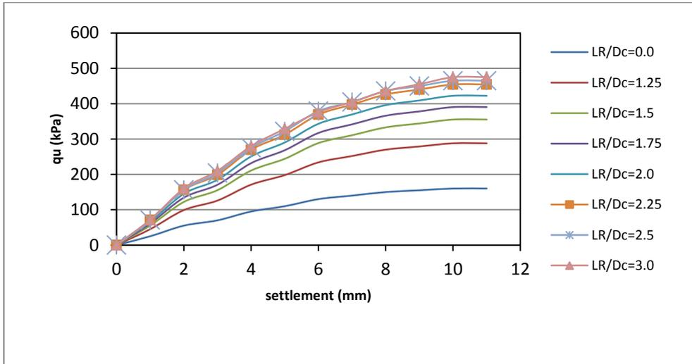
Figure (6): Ultimate bearing pressure – settlement curves for  $D_f/D_c=1.0$ ,  $RD=60\%$
