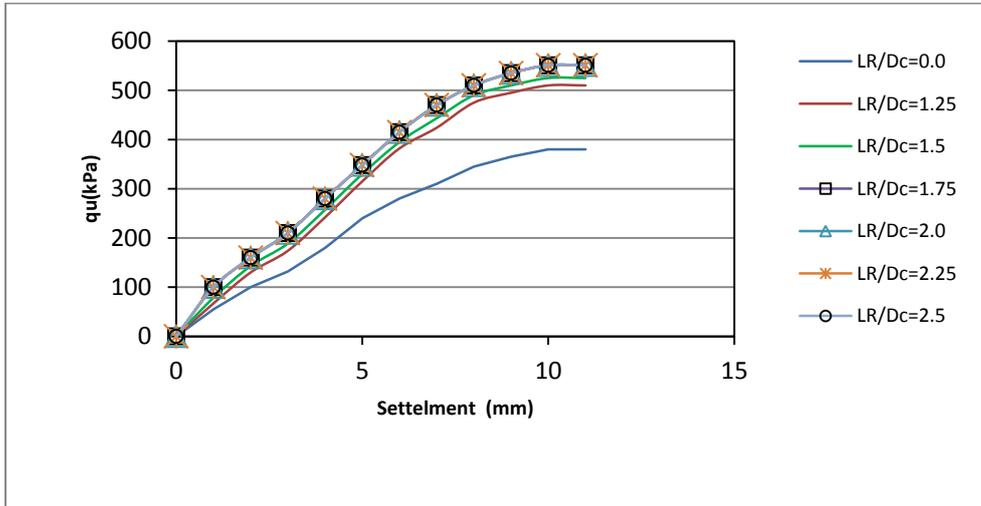
Figure (9): Ultimate bearing pressure – settlement curves for  $D_f/D_c=1.0$ ,  $RD=80\%$
