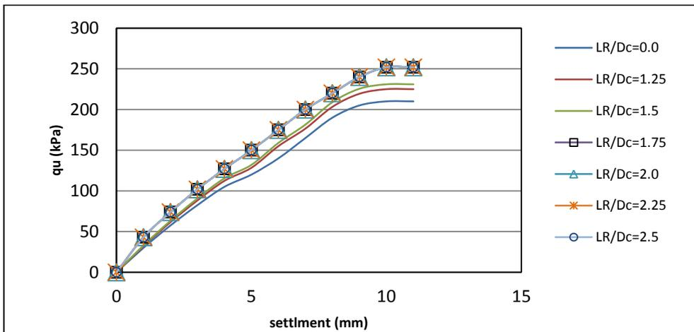
Figure (7): Ultimate bearing pressure – settlement curves for  $D_f/D_c=0.0$ ,  $RD=80\%$
