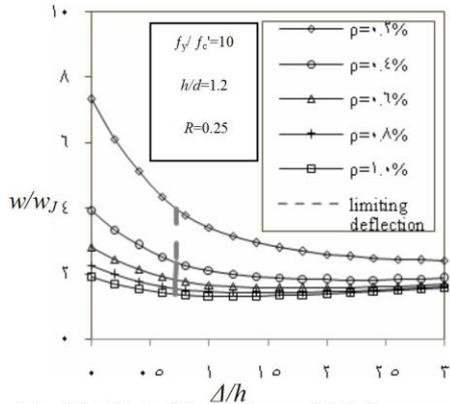
Fig. (8) Effect of Percentage of Reinforcement on  $w/w_J$
