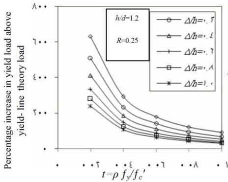
Fig. (10) Variation of the Percentage Increase in the Yield Load above Yield - Line Theory Collapse Load with the Parameter ( $t$ ) for Different Values of  $\Delta/h$
