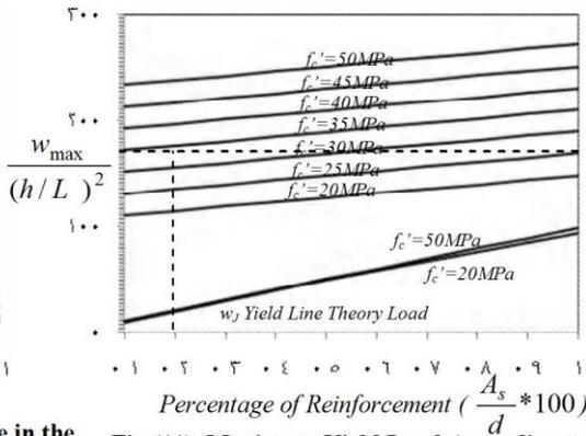
Fig. (11) Maximum Yield Load According to Rigid-Plastic Theory
