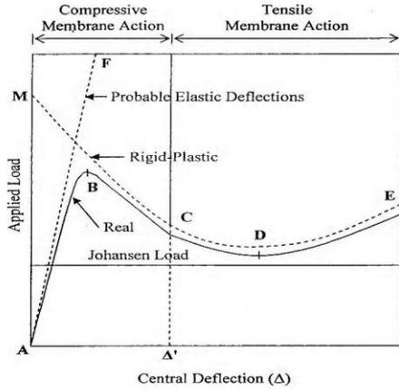
Fig. (1) Load-Deflection Relations for Laterally Restrained R.C Slabs (Reference 3)
