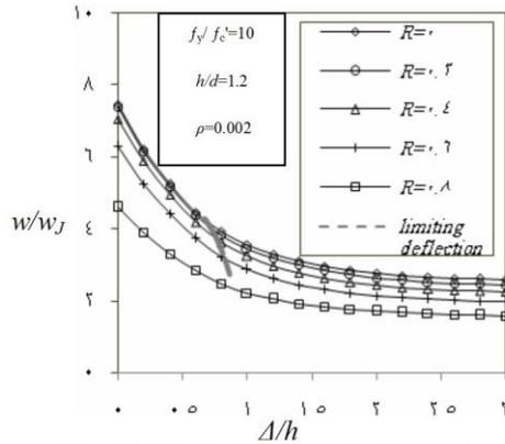
Fig. (9) Effect of Opening Ratio on  $w/w_J$
