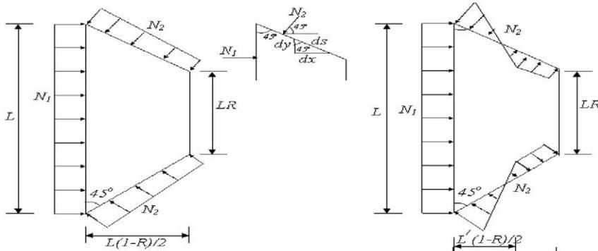
(a) Before the Formation of a Pure Tensile Membrane
