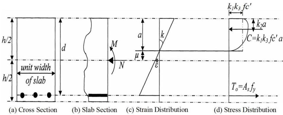
Fig. (2) Stress Distribution on a Slab Section at Yield
