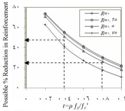
Fig. (13) Practical Significance of Considering Membrane Action in Slab Design
