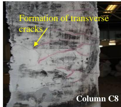
**Figure (14):** SCC column exposure to fire 700°C and eccentric loading.
