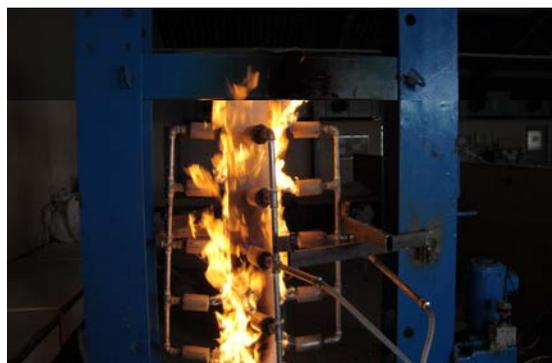
**Figure (6): Testing of SCC column under 15% of ultimate load with exposure burning.**
