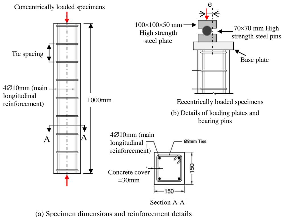
**Figure (2): Specimen details and loading plate arrangement.**
