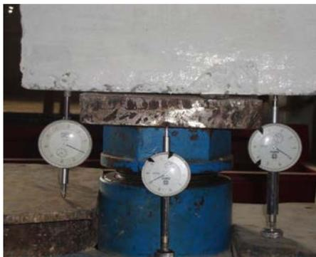
**Figure (5): Testing measurement of axial deformation.**
