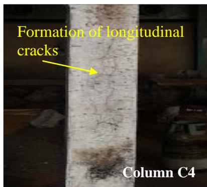
**Figure (13):** SCC column exposure to fire 400°C and concentric loading.
