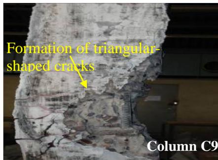
**Figure (15):** SCC column exposure to fire 700°C and eccentric loading prior to failure.
