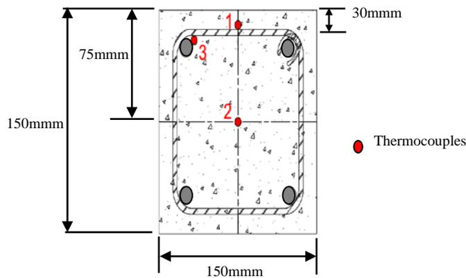
**Figure (7): Thermocouples locations at midheight section in model SC columns.**
