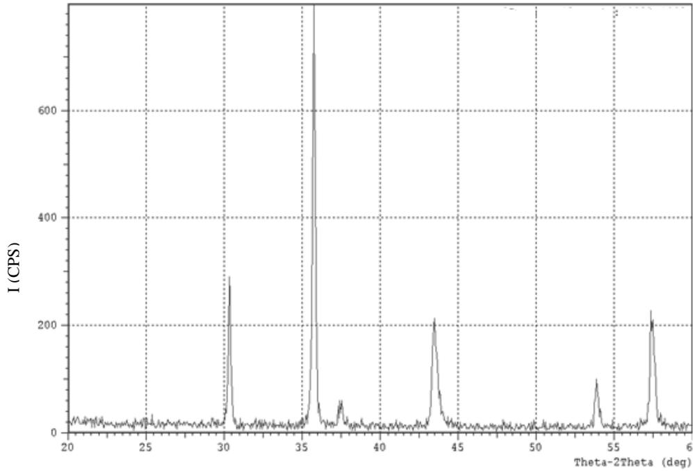
**Figure (1): XRD pattern of the prepared lithium-ferrite powder at 800 °C.**
