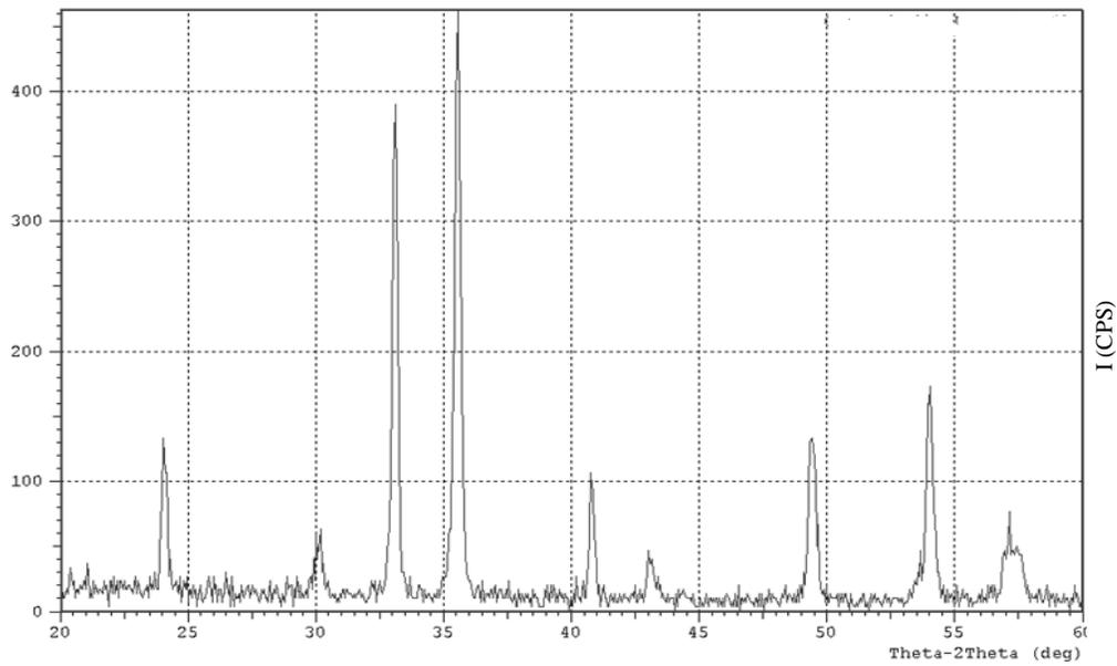
**Figure (2): XRD pattern of the prepared cobalt-ferrite powder at 800 °C.**
