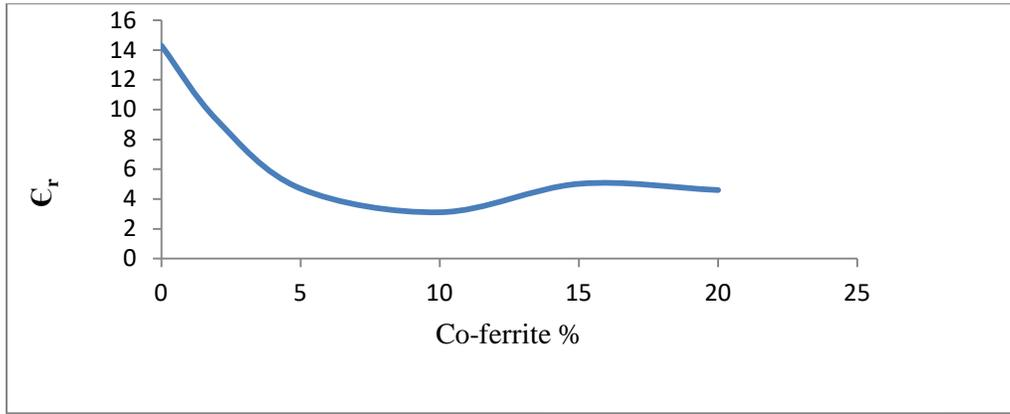
Figure(8): The dielectric constant of lithium-ferrite with different percentage of cobalt-ferrite at 1MHz.
