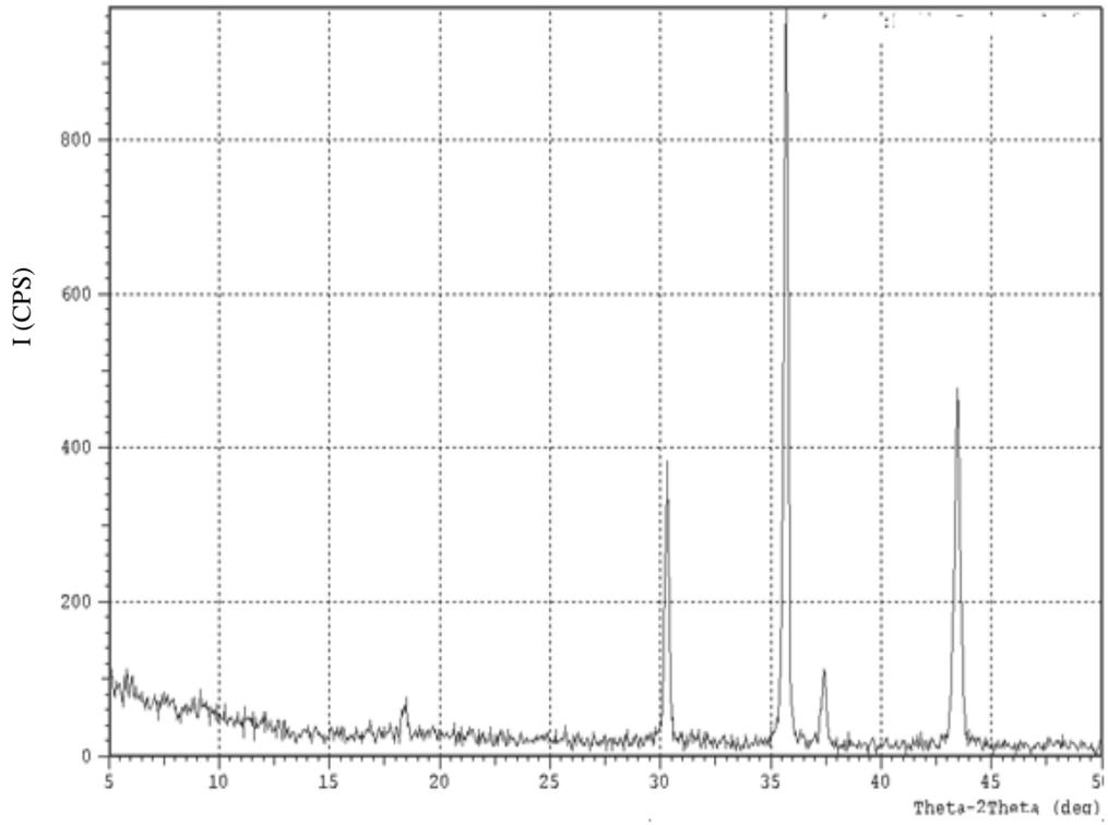
**Figure (5): XRD pattern of lithium-ferrite doped with 20% cobalt-ferrite at 800°C.**
