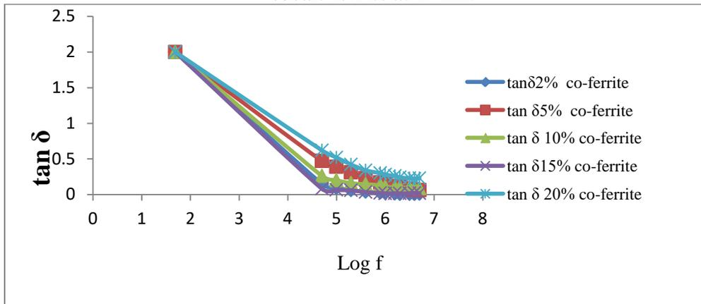
Figure (9): The relation between loss tangent ( $\tan \delta$ ) and frequency of lithium-ferrite with different percentage of cobalt-ferrite.
