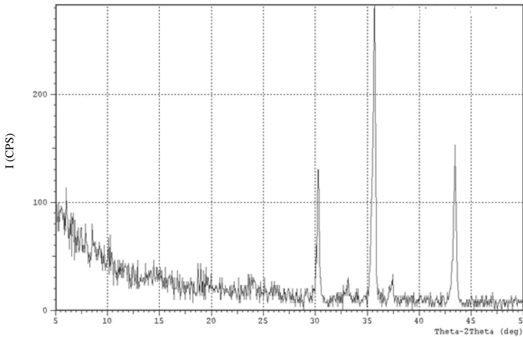
Figure (4): XRD pattern of lithium-ferrite doped with 10% cobalt-ferrite at 800 °C.
