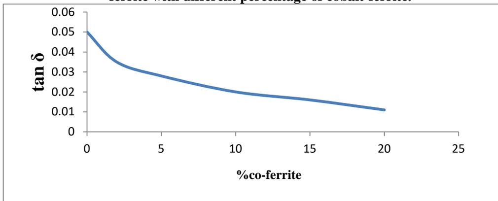
Figure (10): The loss tangent ( $\tan \delta$ ) of lithium-ferrite with different percentage of cobalt-ferrite at 1MHz.
