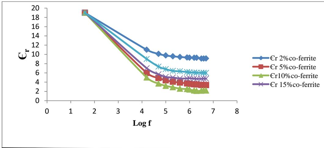
Figure (7): The relation between dielectric constant and frequency of lithium-ferrite with different percentage of cobalt-ferrite.
