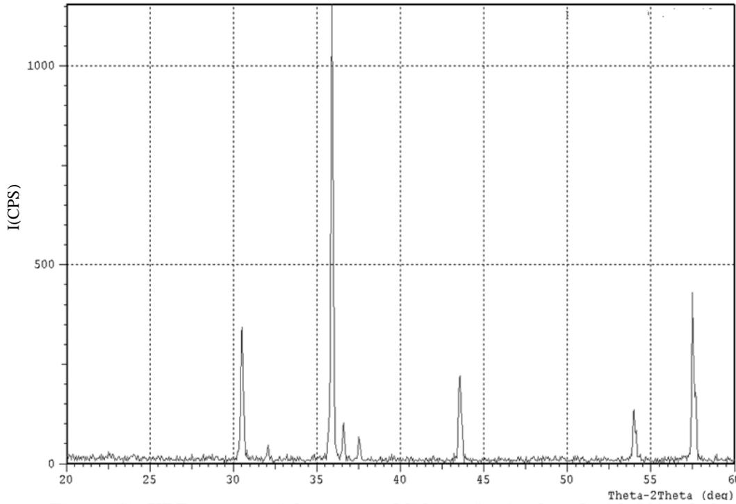
Figure (3): XRD pattern of the prepared lithium ferrite doped with 2% cobalt-ferrite at 800 °C.
