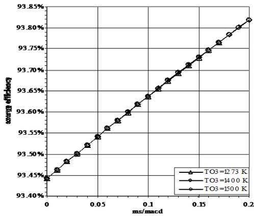
Fig. (10) Change in compressor exergy efficiency due to change in turbine inlet temperature
