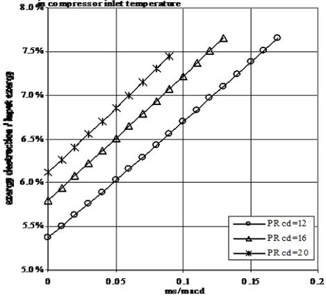
Fig. (19) Change in turbine exergy destruction due to change in compressor design pressure ratio
