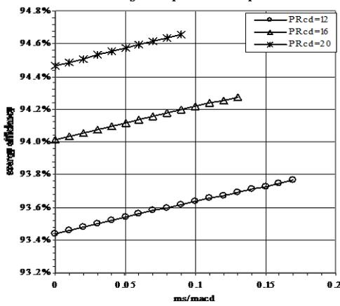
Fig. (8) Change in compressor exergy efficiency due to change in design compressor pressure ratio
