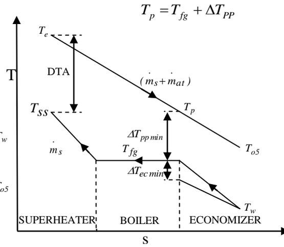
**Fig.(3) Schematic diagram of HRSG components. temperature profile.**
