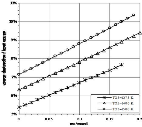
Fig. (21) Change in turbine exergy destruction due to change in turbine inlet temperature
