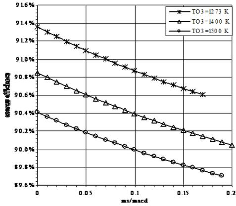
Fig. (22) Change in turbine exergy efficiency due to change in turbine inlet temperature
