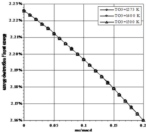
Fig. (9) Change in compressor exergy destruction due to change in turbine inlet temperature
