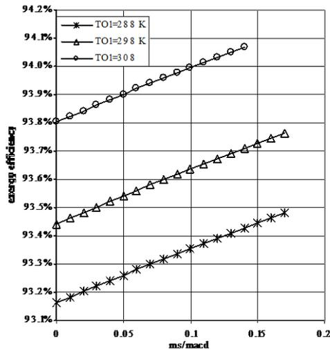
Fig. (6) Change in compressor exergy efficiency due to change in compressor inlet temperature
