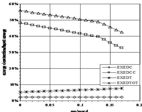
Fig.(23) Exergy destruction comparison for gas turbine components
