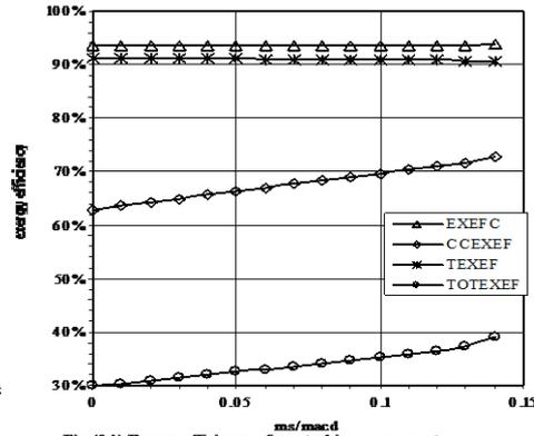
Fig.(24) Exergy efficiency of gas turbine components
