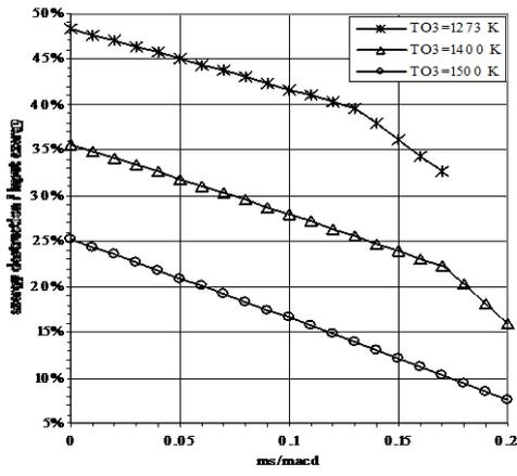
Fig. (15) Change in combustion chamber exergy destruction due to change in turbine inlet temperature
