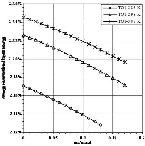
Fig. (5) Change in compressor exergy destruction due to change in compressor inlet temperature
