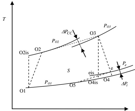
Fig.(1) Single-shaft engine with HRSG.
