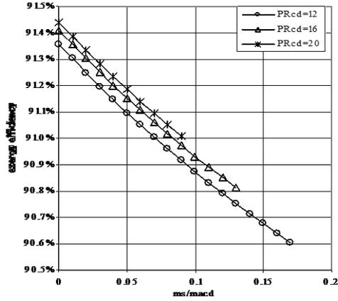
Fig. (20) Change in turbine exergy efficiency due to change in design compressor pressure ratio
