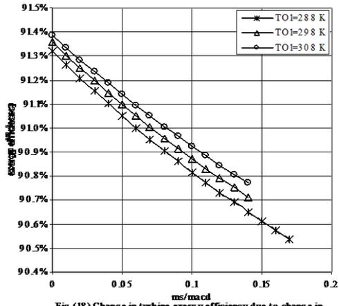
Fig. (18) Change in turbine exergy efficiency due to change in compressor inlet temperature
