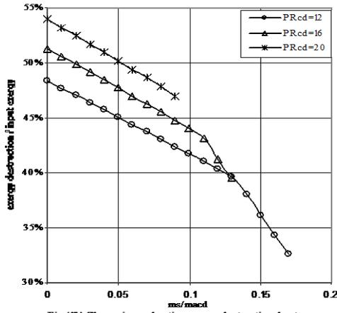
Fig. (13) Change in combustion chamber exergy destruction due to change in compressor pressure ratio
