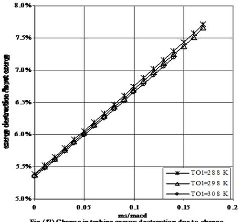
Fig. (17) Change in turbine exergy destruction due to change in compressor inlet temperature
