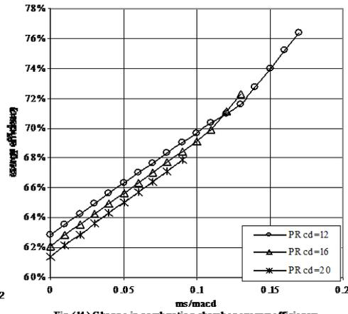
Fig. (14) Change in combustion chamber exergy efficiency due to change in compressor pressure ratio
