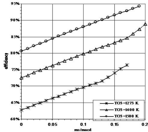
Fig. (16) Change in combustion chamber exergy efficiency due to change in turbine inlet temperature
