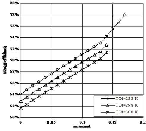
Fig. (12) Change in combustion chamber exergy efficiency due to change in compressor inlet temperature
