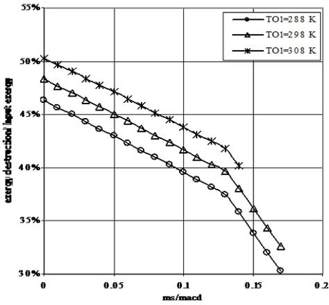
Fig. (11) Change in combustion chamber exergy destruction due to change in compressor inlet temperature
