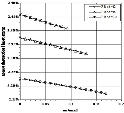
Fig. (7) Change in compressor exergy destruction due to change in design compressor pressure ratio
