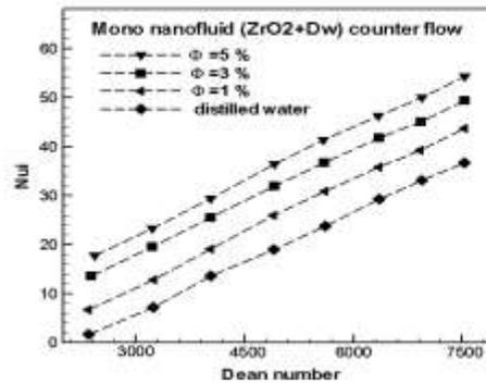
Figure (12). Change of inner Nusselt number for Mono Nano fluid (ZrO<sub>2</sub>+Dw) with counter flow
