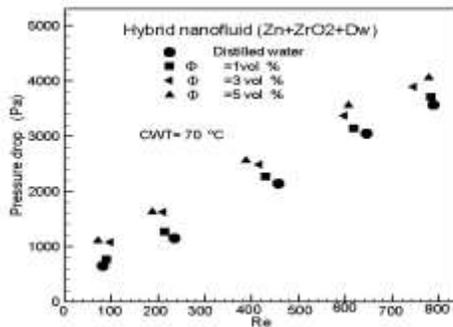
Figure(17). Pressure drop versus Re to hybrid Nano fluid (Zn +ZrO<sub>2</sub>+ Dw) with counter flow at different  $\Phi$
