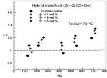
Figure (20) The performance index versus Re to hybrid Nano fluid (Zn+ZrO<sub>2</sub> + Dw) with counter flow at different  $\Phi$
