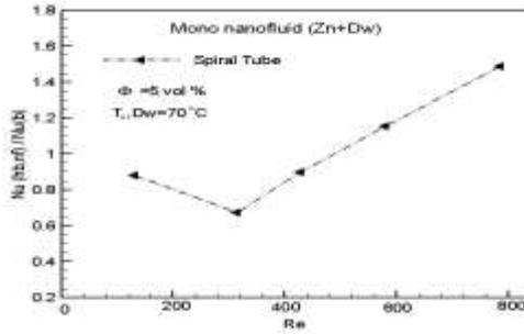
Figure (13) The Nu ratio versus Re to Mono Nano fluid (Zn+ Dw) in spiral tube at  $\Phi=5$  vol %
