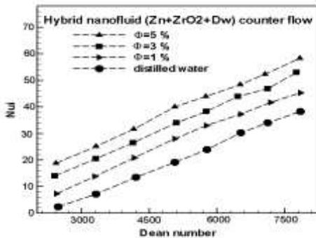
Figure (11). Change of inner Nusselt number for hybrid Nano fluid (Zn+ZrO<sub>2</sub>+Dw) with counter flow
