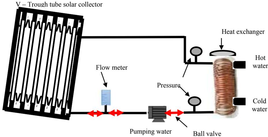
Figure (3) The experimental set up schematic
