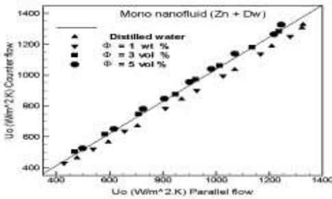
Figure(7). Comparison of  $U_0$  of counter and parallel flow configuration (Zn +Dw) Mono Nano fluid
