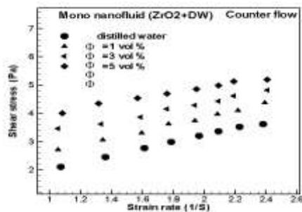
Figure.(24). Shear stress versus shear rate for mono Nano fluid (ZrO<sub>2</sub>+Dw) flow with counter
