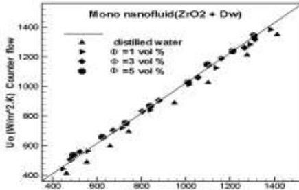
Figure (9). Comparison of  $U_0$  of counter and parallel flow configuration (ZrO<sub>2</sub>+ Dw) Mono Nano fluid
