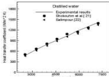
Figure( 5). Comparison between calculated and measured heat transfer coefficient of Dw [21,22]
