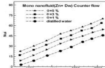
Figure (10). Change of inner Nusselt number for Mono Nano fluid (Zn+Dw) with counter flow
