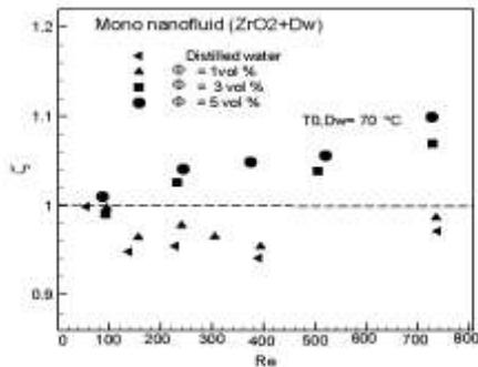
Figure (21) The performance index versus Re to mono Nano fluid (ZrO<sub>2</sub> + Dw) with counter flow at different  $\Phi$
