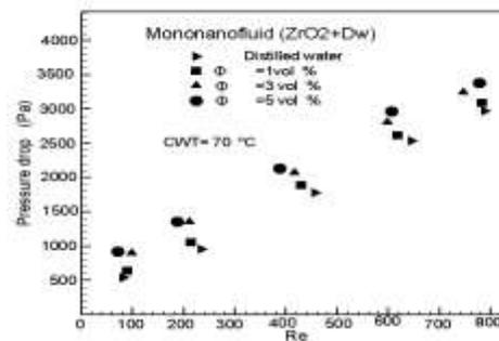
Figure(18). Pressure drop versus Re to Mono Nano fluid (ZrO<sub>2</sub>+ Dw) with counter flow at different  $\Phi$
