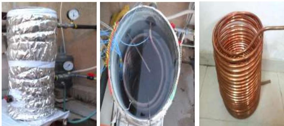
Figure (2) Stages of building heat exchanger
