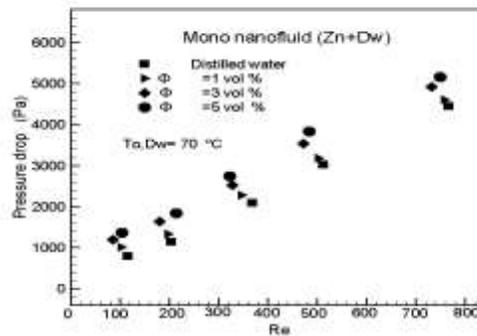
Figure (16) Pressure drop versus Re to Mono Nano fluid (Zn + Dw) with counter flow at different  $\Phi$
