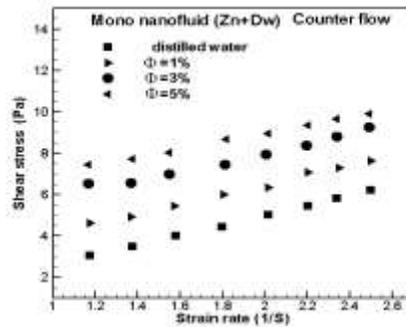
Figure.(22). Shear stress versus shear rate for mono Nano fluid (Zn+Dw) with counter flow
