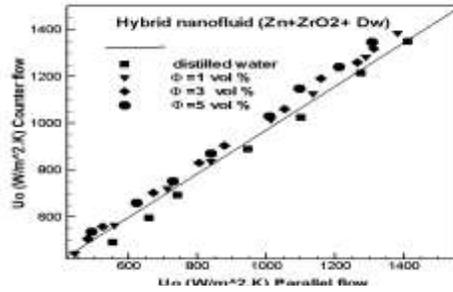
Figure(8). Comparison of  $U_0$  of counter and parallel flow configuration for (Zn +ZrO<sub>2</sub>+ Dw) Hybrid Nano fluid
