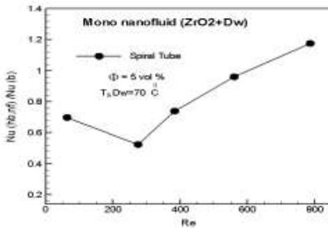
Figure (15) The Nu ratio versus Re to Mono Nano fluid (ZrO<sub>2</sub> + Dw) in spiral tube at  $\Phi=5$  vol%
