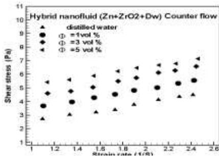
Figure. (23) Shear stress versus shear rate for hybrid Nano fluid (Zn+ZrO<sub>2</sub>+ Dw) with counter flow
