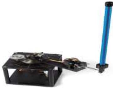
Figure (1) Quanser rotary inverted Pendulum
