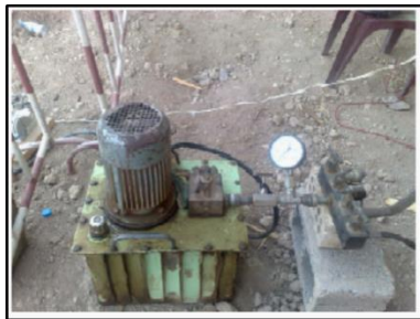
a. Load gauge controlling the load increments and decrements
