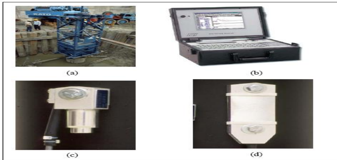
Figure (1): Test Equipment a) 30 tone steel ram with hydraulic release b) Pile Driving Analyzer c) accelerometer d) transducer.
