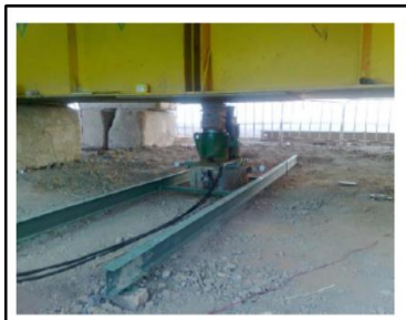
b. Setting the hydraulic jack and displacement gauges over the pile
