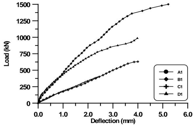
**Figure (17) Effect of UHPC layer thickness on load-deflection of Deep beams with ( $V_f=0.5\%$ )**
