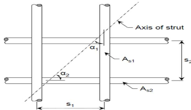
Figure 21: Calculation of web reinforcement in ACI 318-11<sup>[17]</sup>
