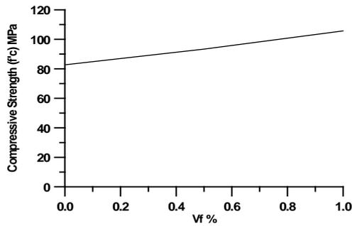
**Figure (8) Effect of steel fibers ratio on compressive strength of UHPC.**
