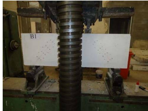
**Figure (7) Deep beam inside machine**
