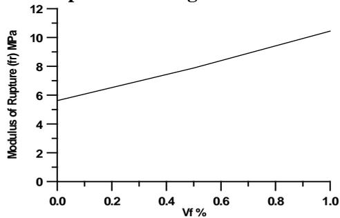
**Figure (10) Effect of steel fibers ratio on modulus of rupture of UHPC.**
