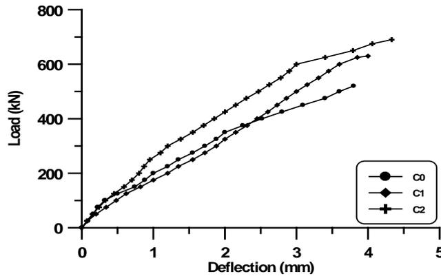
**Figure (14) Load-Deflection Relationship of Hybrid Deep Beams ( $h_R/h=0.25$ )**
