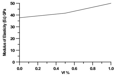
**Figure (9) Effect of steel fibers ratio on modulus of elasticity of UHPC.**
