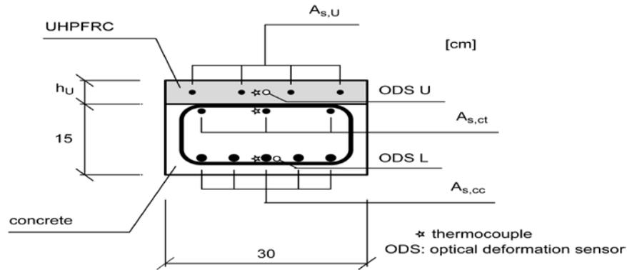
**Figure (1) Cross-section of the composite “UHPFRC-concrete” beams <sup>[15]</sup>**
