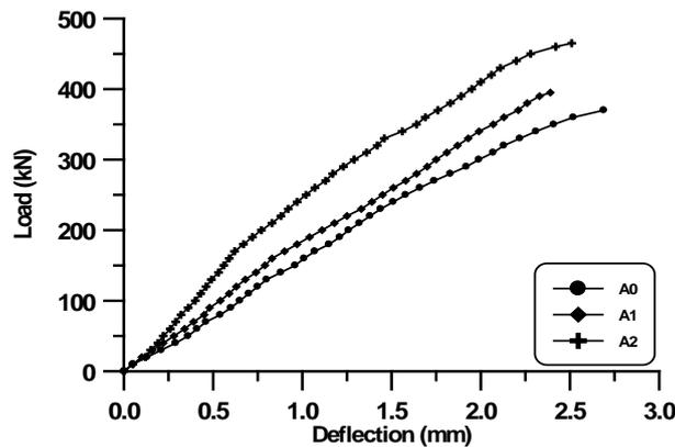
Figure (12) Load-Deflection Relationship of CC Deep Beams
