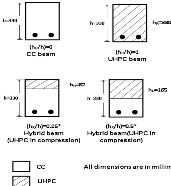
**Figure (5) Types of the tested beams**
