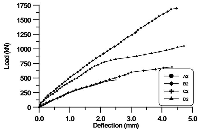
**Figure (18) Effect of UHPC layer thickness on load-deflection of Deep beams with ( $V_f=1\%$ )**
