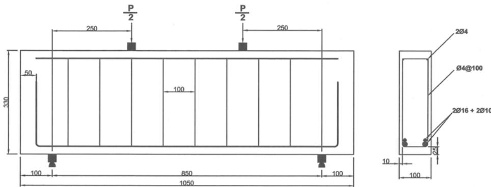
**Figure (4) Typical dimensions (mm) and details of tested deep beam**
