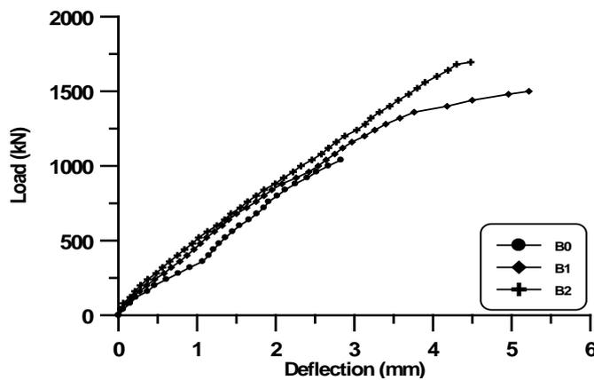
Figure (13) Load-Deflection Relationship of UHPC(hR/h=1) Deep Beams
