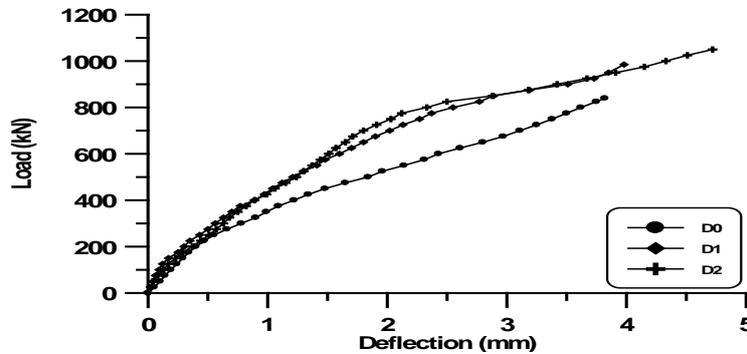
**Figure (15) Load-Deflection Relationship of Hybrid Deep Beams ( $h_R/h=0.5$ )**
