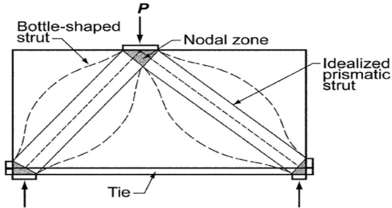
Figure 20: Shape of strut<sup>[17]</sup>
