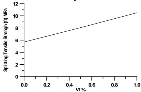
**Figure (11) Effect of steel fibers ratio on splitting tensile strength of UHPC.**
