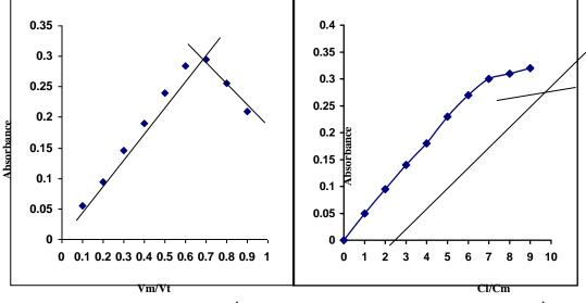
(a) Job's [promethazine.HCl( $3.116 \times 10^4 \text{ M}$ ) / (b) Mole ratio [ promethazine.HCl( $3.116 \times 10^4 \text{ M}$ )] promethazine.HCl+In (III) ( $3.116 \times 10^4 \text{ M}$ )] /In (III) ( $3.116 \times 10^4 \text{ M}$ )]
