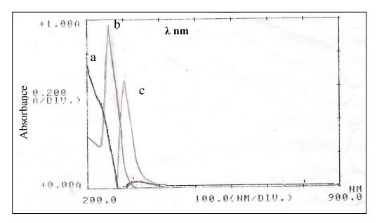
Figure 1: Absorption spectra of (a)50  $\mu$ g/ml of In(III) (b)200  $\mu$ g/ml of promethazine. HCl (c) 200  $\mu$ g/ml of promethazine HCl with 50  $\mu$ g/ml of In (III) against reagent blank.
