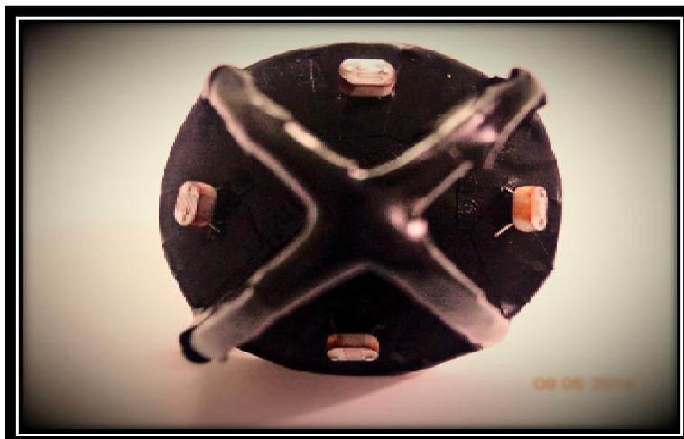
**Figure (3) Four LDR sensors used to detect the sun light**
