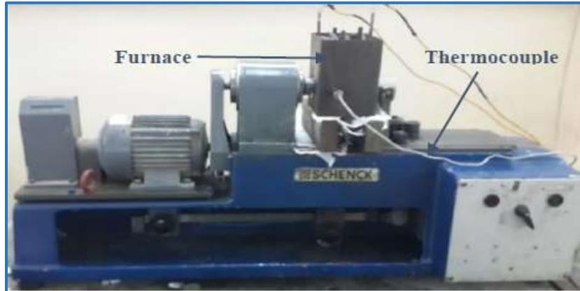
Figure (3) Furnace attached to fatigue machine.
