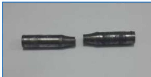
**Figure (2). Fatigue test specimen after fracture.**
