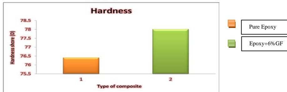
**Figure (15) Hardness shore (D) of pure epoxy and epoxy +6% glass fiber**
