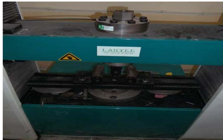
**Figure (8): Flexural strength and shear stress device**
