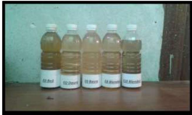
Figure (3): Pure diesel and the ethanol blend samples
