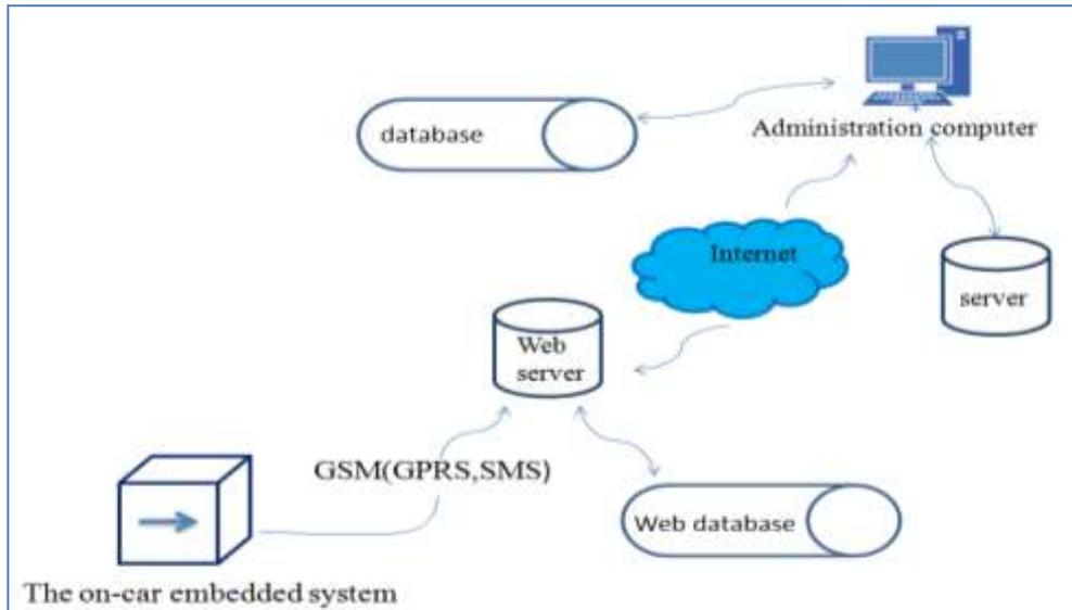
Figure (1) System design architecture
