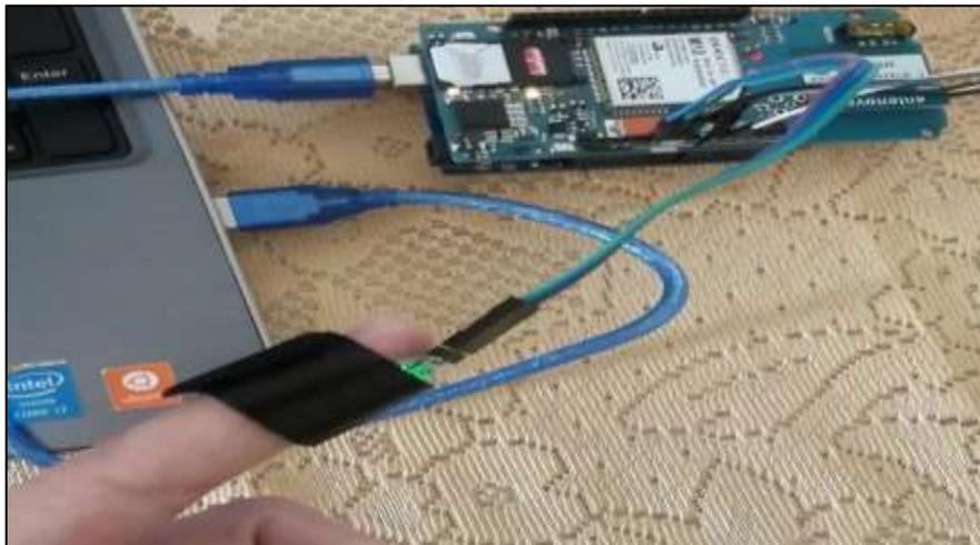
Figure(17) Arduino Uno and GSM Arduino shield to send vital sign data for patient.
