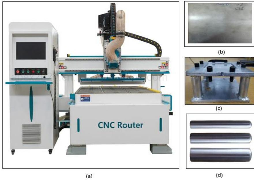
**Fig. 1. a) CNC milling machine b) Base sheet of pure titanium c) Fixture d) Tools.**
