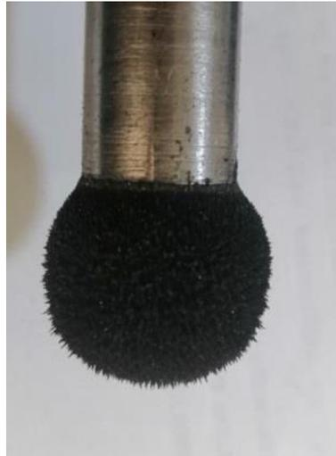
**Fig. 4. Accumulation of powder on the tool.**
