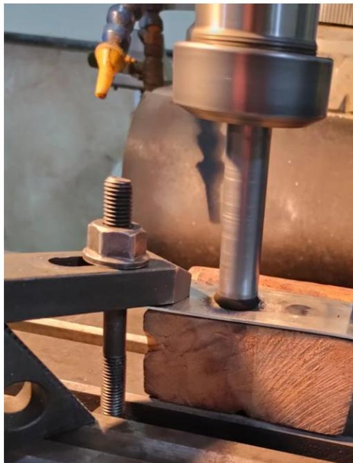
**Fig. 3. Experimental setup of MAF tool.**
