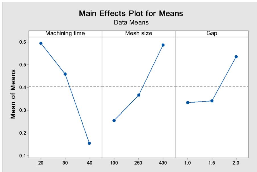
Fig. 5. Main effect plot of surface roughness.
