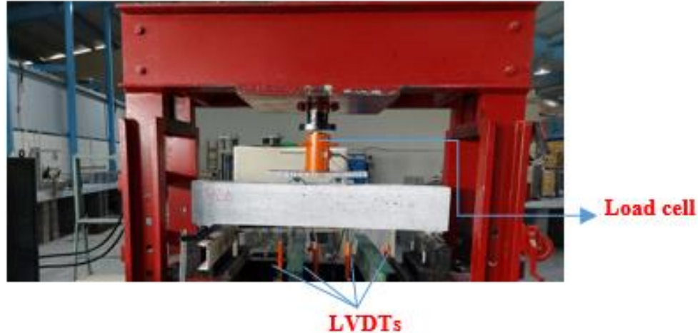
Fig. 2 Actual beam specimen under testing
