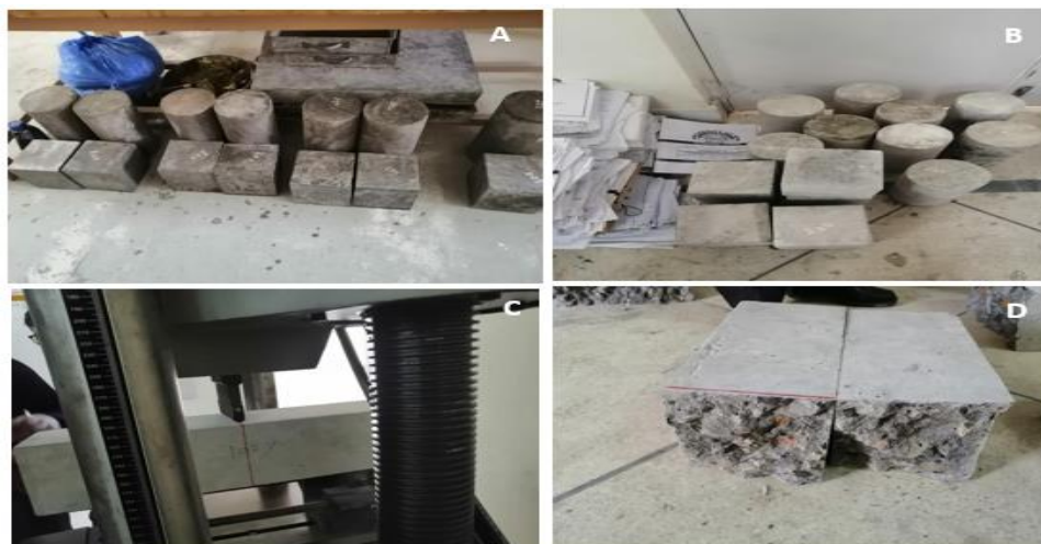
Fig. 7 Blocks and Cylinder specimens for Compressive, Tensile, and Flexural strength test
