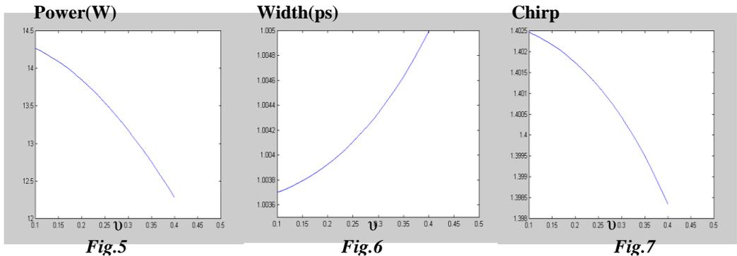
**Fig. (5,6and7).** The power P, width and chirp of soliton as a function of different values of  $\nu$  respectively.
