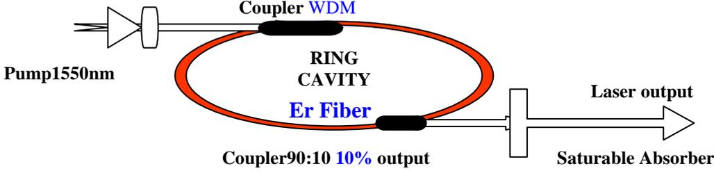
Fig. (3) schematic diagram for theoretical model WDM, wavelength division multiplexer.
