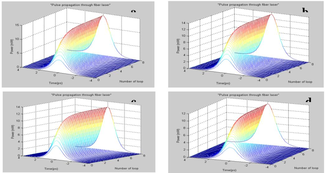
**Fig. 8.** Evolution toward the steady-state soliton over 4 loops for  $\gamma=0.02\text{Wm}^{-1}$   $\alpha=0.1\text{db}\backslash\text{m}^{-1}$   $\delta=0.1$ ,  $B_2=-0.01\text{ps}^2/\text{m}$ ,  $\nu=0.1$  and  $\tau=1\text{ps}$  (a)  $\zeta=0.1$  (b)  $\zeta=0.2$  (c)  $\zeta=0.4$  (d)  $\zeta=0.6$ .
