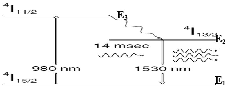
**Fig. 1 Energy-levels of Erbium in Silica Glass**
