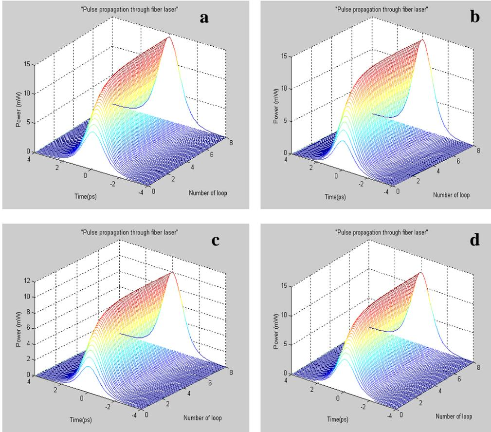
**Fig. 4.** Evolution toward the steady-state soliton over 4 loops for  $\gamma=0.02\text{Wm}^{-1}$ ,  $\alpha=0.1\text{dBm}^{-1}$ ,  $\delta=0.1$ ,  $B_2=-0.01\text{ps}^2/\text{m}$ ,  $\zeta=0.1$  and  $\tau=1\text{ps}$  (a)  $v=0.1$  (b)  $v=0.2$  (c)  $v=0.4$  (d)  $v=0.6$ .
