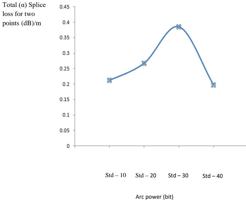
**Figure (9) Splice losses of SMF-PCF as a function of the fusion power when the fusion time is fixed at(1000 ms.)**
