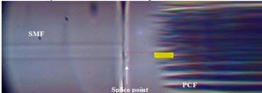
**Figure (11):** Microscope image of the splice zone between PCF (ESM-12) on the right, and the SMF-28 on the left. The collapsed length is ~92.726μm at STD - 30 (bit) and Arc time 1000 ms
