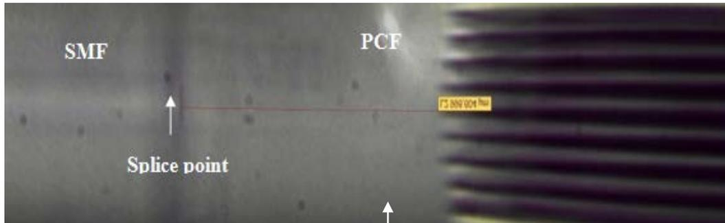
**Figure (10):** Microscope image of the splice zone between PCF (ESM-12) on the right, and the SMF-28 on the left. The collapsed length is ~90.604 at STD - 40 (bit) and Arc time 1000 ms
