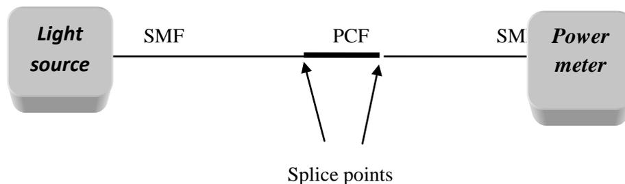
**Figure (3): schematic of splicing (SMF-28/ESM-12/SMF-28)**
