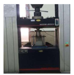
Figure 3A: The deep drawing tools mounted in the testing machine.
