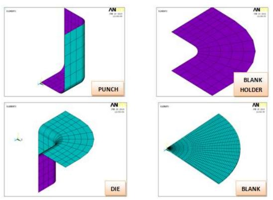
Figure 4: FE model of the sheet material and drawing die parts.
