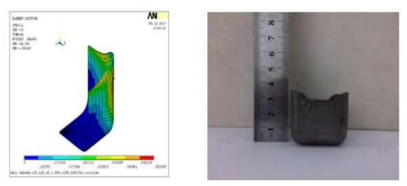
Figure 5: Cup drawn by numerical simulation and experimental.
