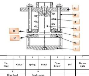
Figure 3B: Schematic representation of rig deep drawing tooling
