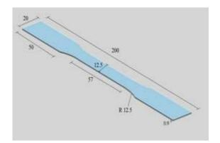
Figure 2: The dimensions of the standard tensile test specimen.
