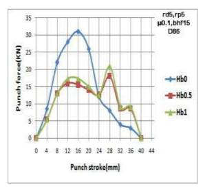
Figure 7: The effect of high draw bead on punch force.
