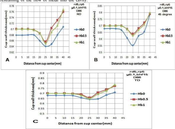
Figure 8: The effect of high draw bead on the cup wall thickness along, A) rolling direction, B) 45° from RD, C) transverse direction.
