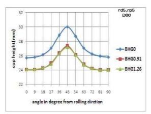
Figure 11: The effect of blank holder gap on the height of cup.
