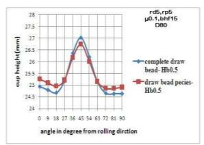
Figure 10: Comparison between complete draw bead around the circumference die surface and pieces draw bead in the 0° and 90° from RD.
