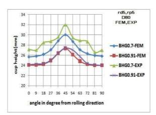
Figure 12: The effect of blank holder gap on cup height (experimental and numerical)
