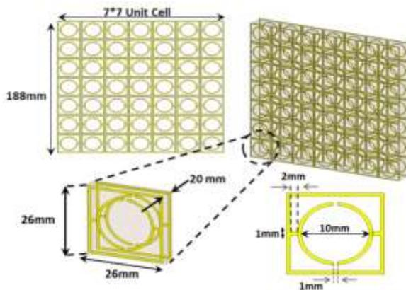
Figure 2: UC-PBG Geometry.
