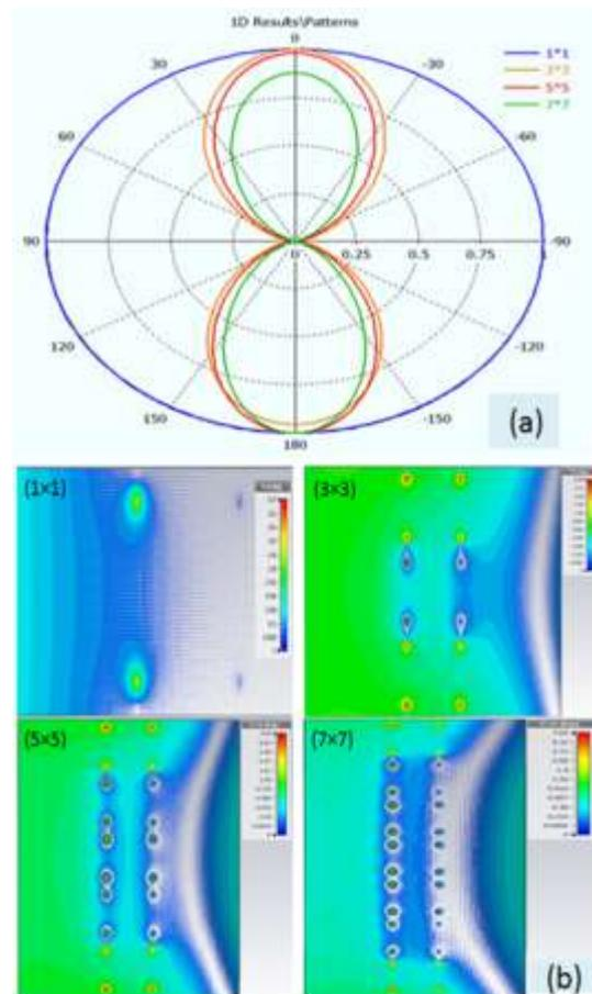
Figure 6: Plane wave results at 915 MHz; (a) 2-D view and (b) 3-D view.
