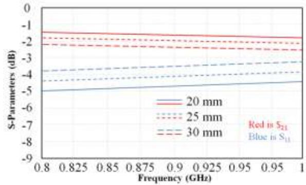
Figure 5: UC-PBG performance regarding S-parameters spectra of the proposed unit cell with different separations distance.
