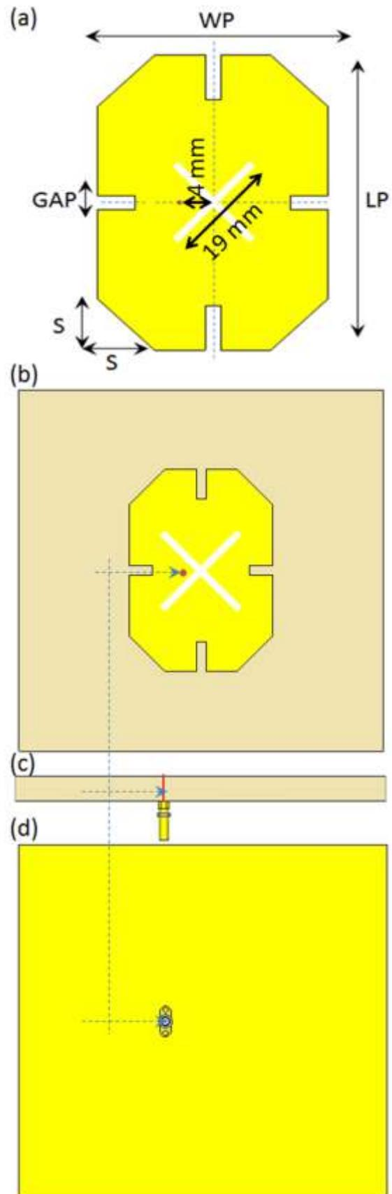
**Figure 1: Antenna geometry: (a) Patch structure, (b) Front view, (c) Side view, (d) Back view.**
