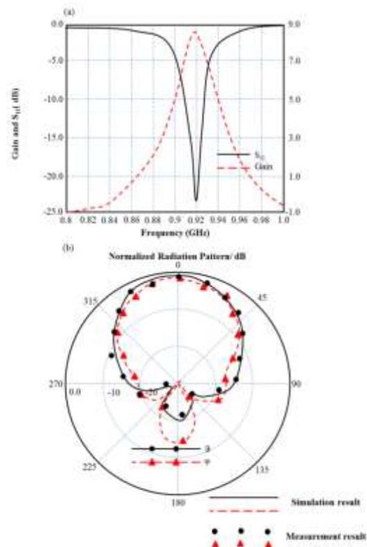
Figure 12: Microstrip antenna based UC-PBG Layers measurements: (a) Gain and  $S_{11}$  spectra and (b) radiation patterns for measured and simulated results.
