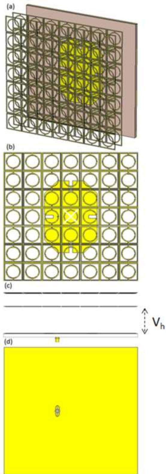
Figure 3: Microstrip antenna based on UC-PBG Layers: (a) 3-D view. (b) The structure front view (c) side view (d) back view.
