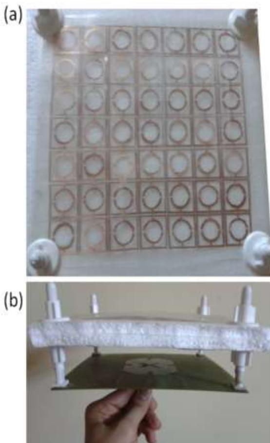
Figure 11: The fabricated prototype with the UC-PBG layers; (a) Top view (b) Side view.
