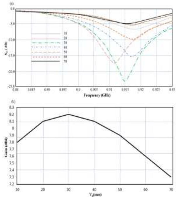
Figure 9: Parametric study of the proposed UC-PBG Layers from the antenna structure: (a)  $S_{11}$  and (b) bore sight gain.
