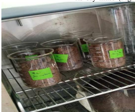
**Figure 2. Dry soil samples in the oven**
