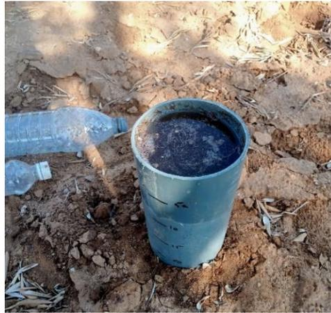
Figure 4. Measurement of infiltration in the normal soil state
