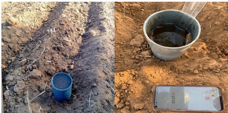
Figure 6. Infiltration at the furrow tilled by plow
