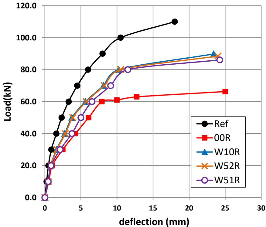
Fig. 9. Comparison load deflection curve for slabs with rectangular openings strengthen with wire mesh.
