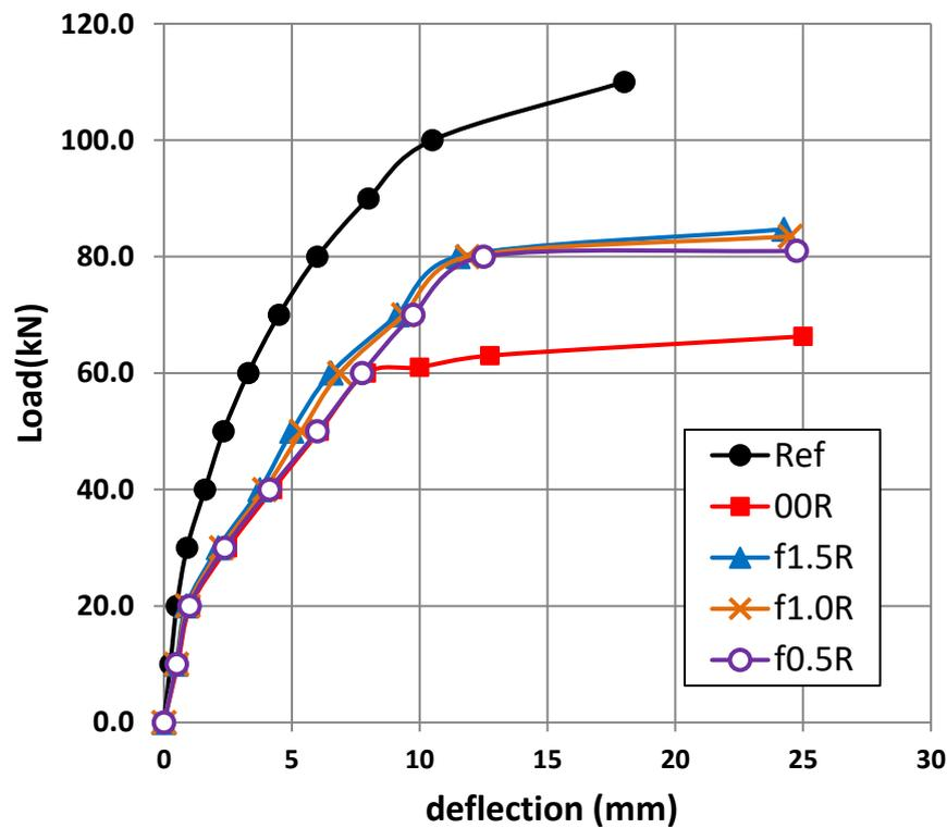
Fig. 8. Comparison load deflection curve for slabs with rectangular openings strengthened with steel fibers.
