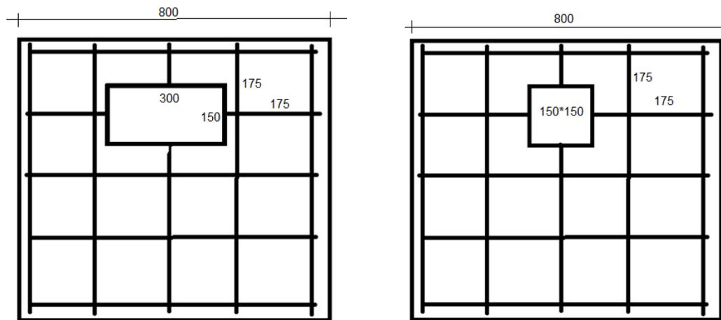
Fig. 1. Details of reinforced concrete slabs with openings.
