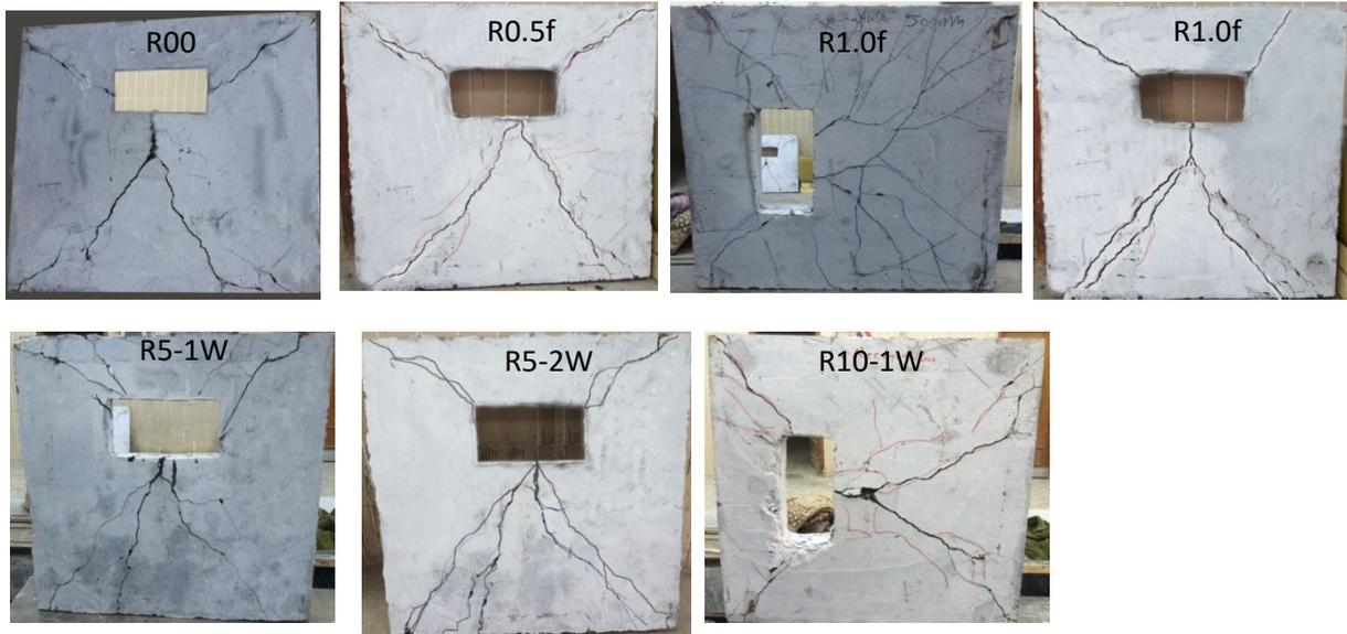
**Fig. 5. Mode of failure and crack pattern of slabs with rectangular openings.**
