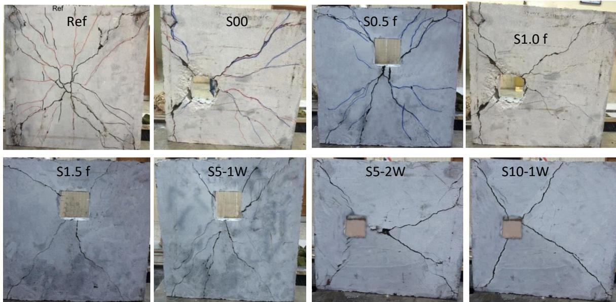
**Fig. 4. Mode of failure and crack pattern of control slab and slabs with square openings.**
