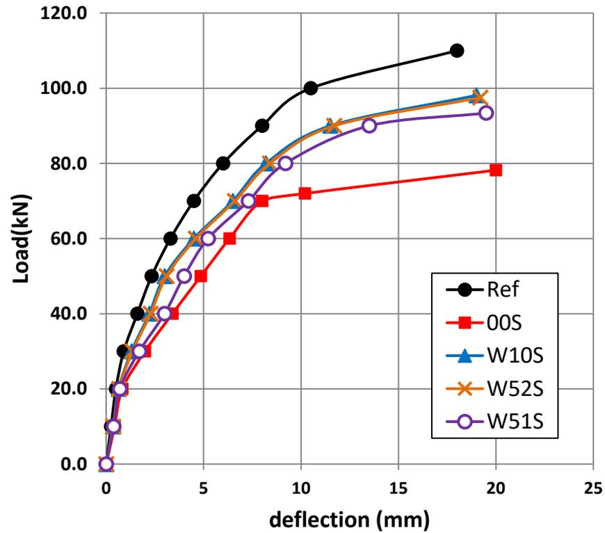
Fig. 7. Comparison load deflection curve for slabs with square openings strengthened with wire mesh.
