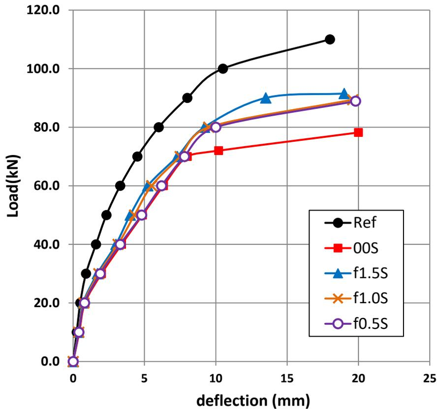
Fig. 6. Comparison load deflection curve for slabs with square openings strengthened with steel fibers.
