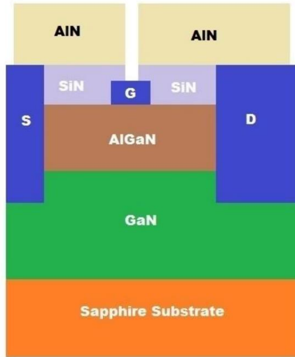
Figure 2: Suggested device design with the AlN layer on top [16].
